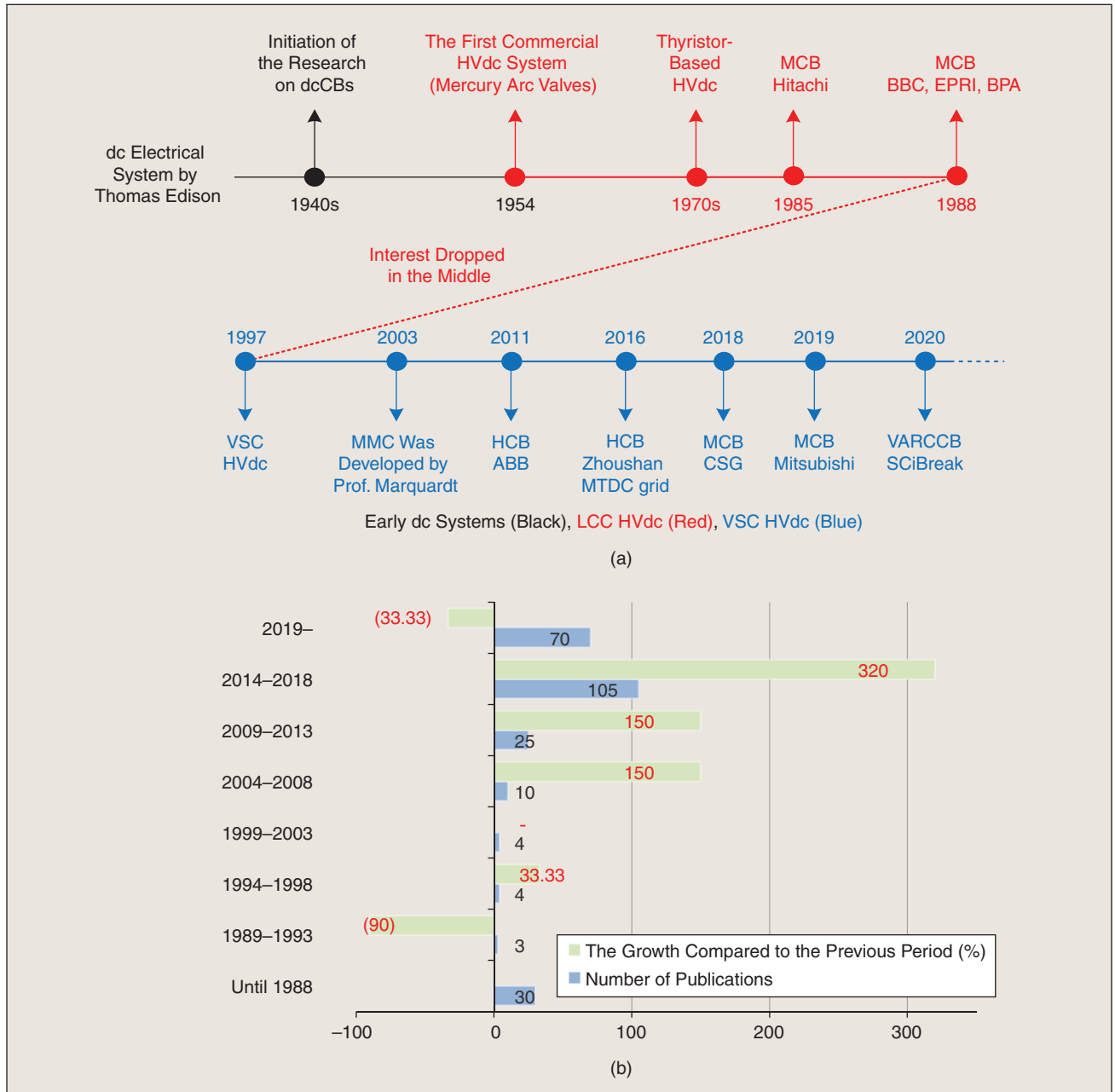
FIGURE 1 – (a) The timeline for the development of dc CBs and (b) the general number of publications on HVdc CBs. MCB: mechanical CB; HCB: hybrid CB; VARCCB: VSC-assisted resonant current CB; MMC: modular multilevel converter; VSC: voltage source converter; CSG: China southern grid; LCC: line-commutated converter; ABB: Asea Brown Boveri Ltd; EPRI: Electric Power Research Institute; BBC: Brown Boveri Company; BPA: Bonneville Power Administration.
