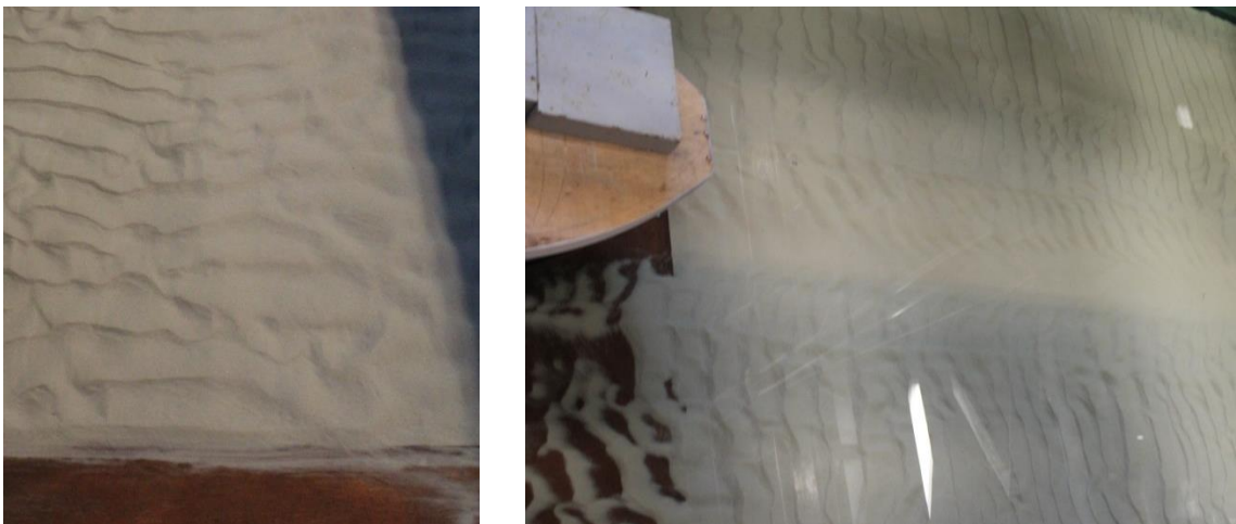
Figure 46: Erosion after experiments with flat bed and a conventional vessel
