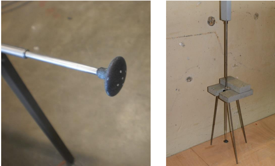
Appendix A - Figure 4: EMS-probe head with electrodes (left) and EMS-30 probe in flume (right)
