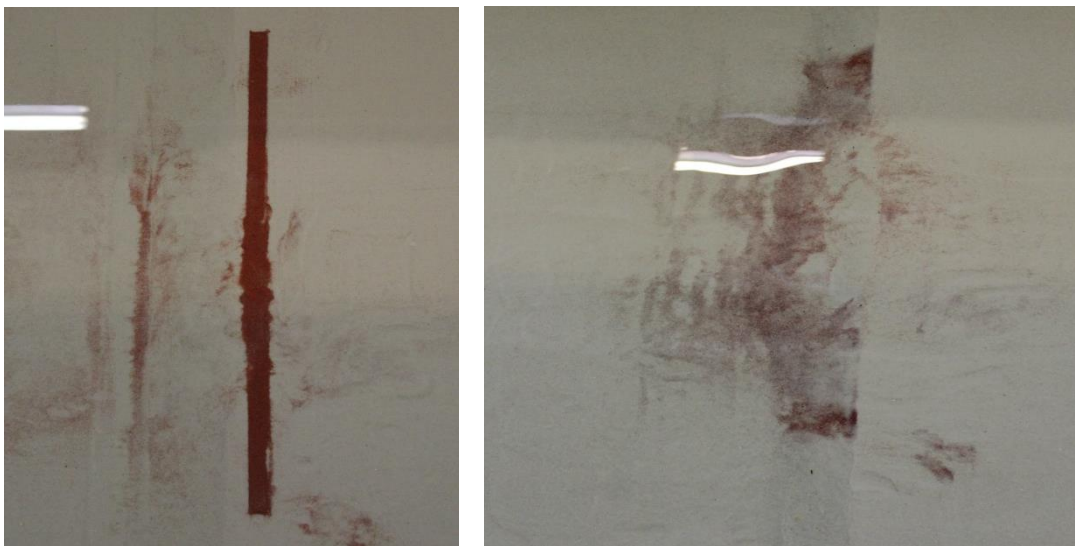
Figure 49: Sediment movement under conventional vessel with dunes (Experiment 51 run 1)
