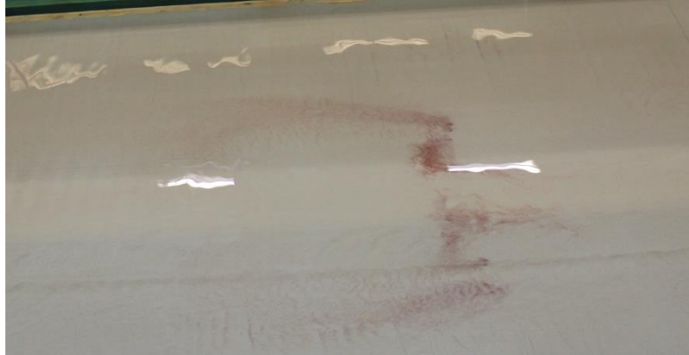
Figure 53: Sediment movement after passage of a barge (Experiment 71 run 1)
