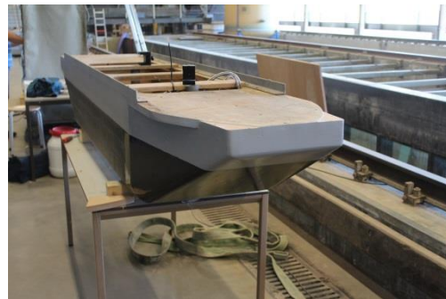
Appendix A - Figure 10: Constructed barge bow
