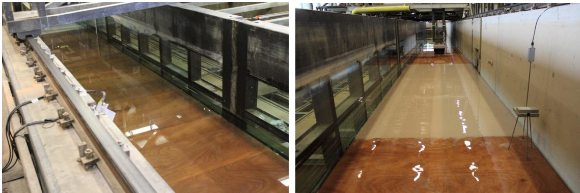
Appendix A - Figure 12: Flat bed without sediment (left) and with sediment (right)
