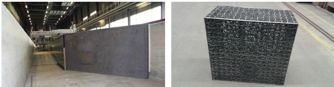
Figure 20: Wave reduction screen (right) and wave energy dissipation box (left)
