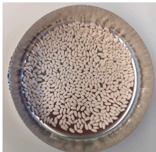
Fig. 1. Printed zeolite granules (after sintering at 950 °C).
