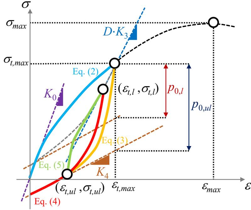
Figure 12: Loading, unloading and reloading branches implemented in the user-supplied subroutine.
