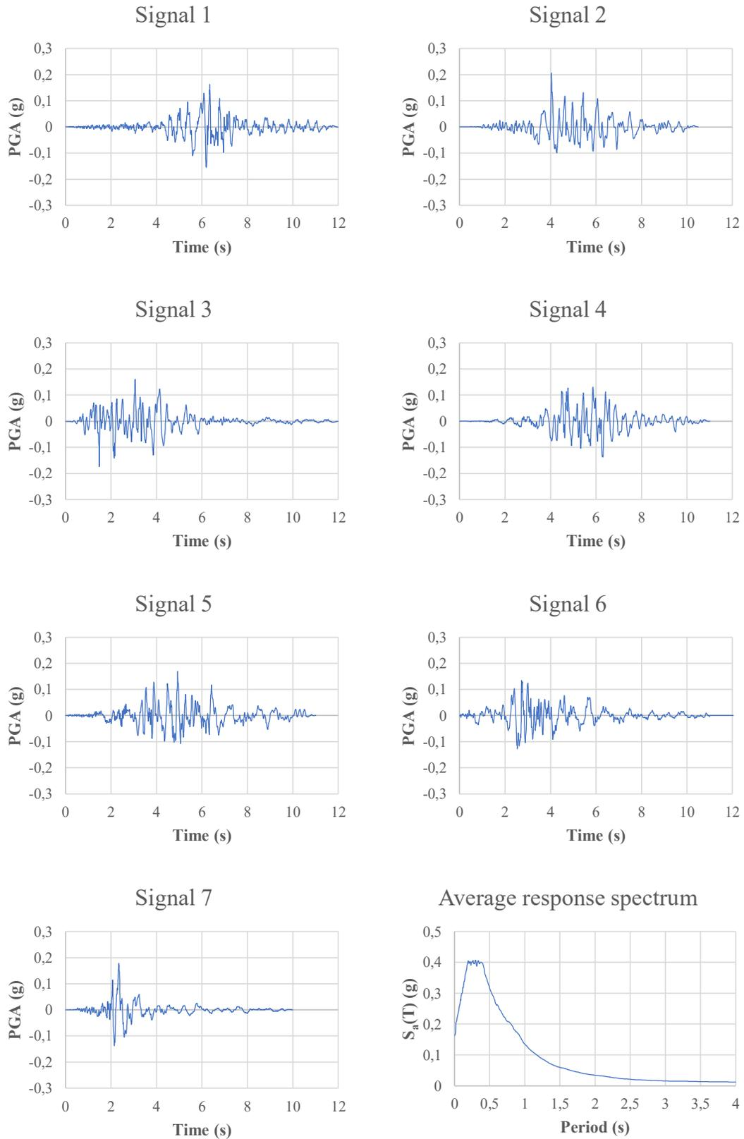
Figure 16: Adopted signals for time-history analyses; their average response spectrum is also reported. Data from NPR 9998 Webtool [35].
