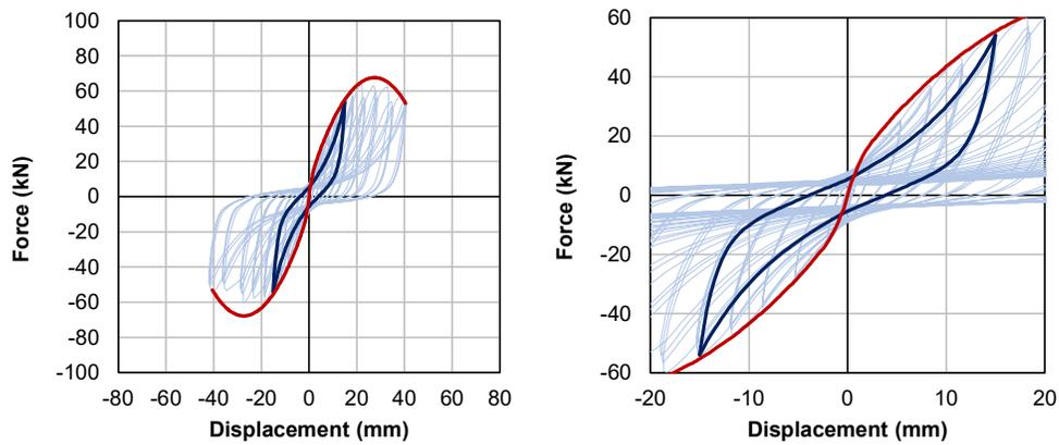
Figure 8: Comparison between analytical backbone (red) and a representative pinching cycle (dark blue) with the experimental hysteretic response (light blue) for sample *DFper-4s*: global (left) and initial (right) response [16].
