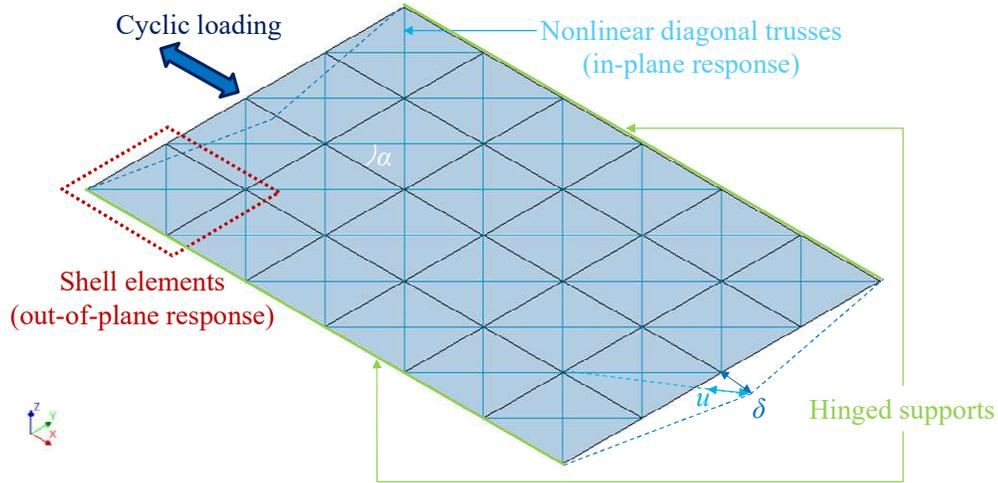
Figure 13: Model of the retrofitted diaphragm for the validation of the user-supplied subroutine.
