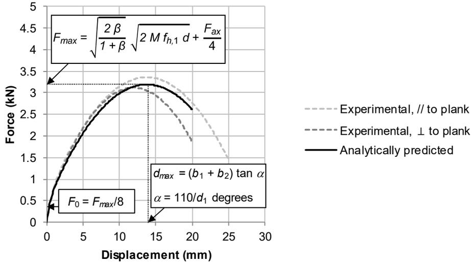
Figure 4: Comparison between the analytically derived curve and the ones obtained from the experimental data [16]. In the reported equations, the same notation as in EN 1995 [22] and EN 409 [24] is used.
