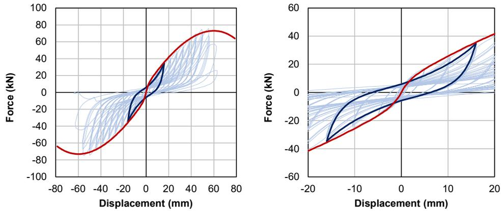
Figure 7: Comparison between analytical backbone (red) and a representative pinching cycle (dark blue) with the experimental hysteretic response (light blue) for sample *DFpar-1s*: global (left) and initial (right) response [16].
