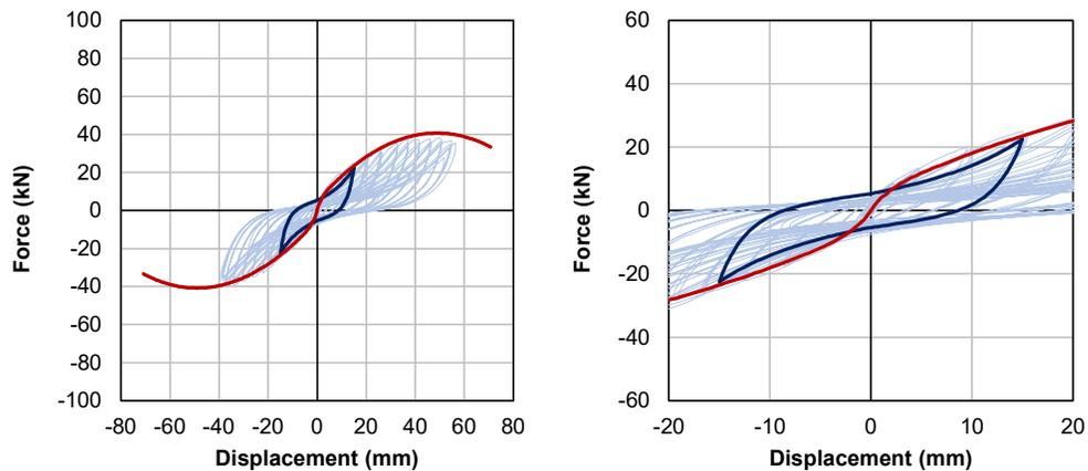
Figure 9: Comparison between analytical backbone (red) and a representative pinching cycle (dark blue) with the experimental hysteretic response (light blue) for sample *DFpar-5s*: global (left) and initial (right) response [16].
