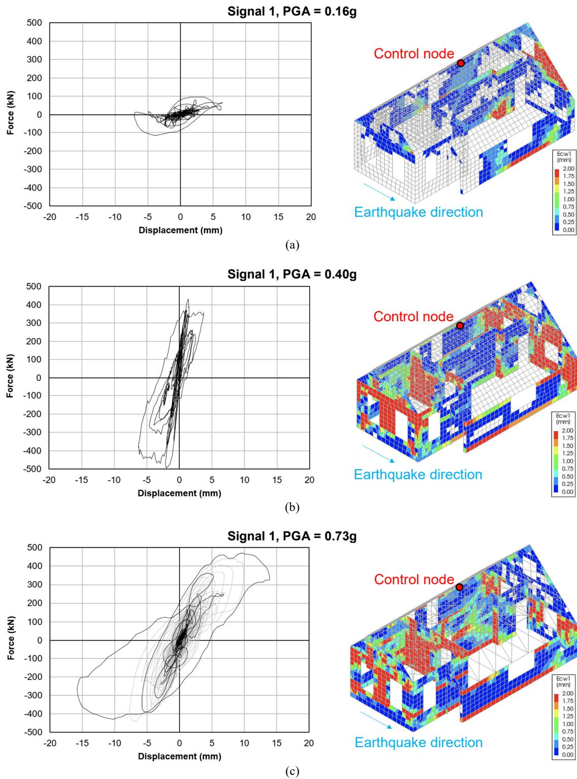
Figure 18: Base shear vs. roof displacement response and crack opening (E<sub>cw1</sub>) pattern of the three configurations: as-built (a), floors strengthened with concrete slabs (b), diaphragms retrofitted with plywood panels (c).
