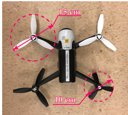
Figure 12: A Bebop 2 quadrotor with one damaged rotor.
