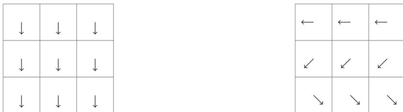
(a) The direction of  $M_{xy}(\mathbf{r}, t)$  caused by the spins on different  $(x, y)$  positions in the selected slice. (b) The influence on the left image after the  $y$ -gradient has quickly been switched on and off.
