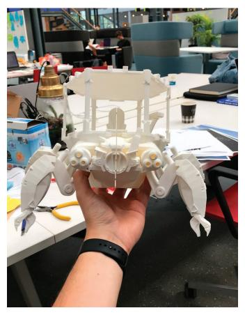
The seams between different parts and some 3D printing inaccuracies were filled with filler, followed by more sanding after drying. Creating a 3D printed model is tedious, but it pays off in the end.
