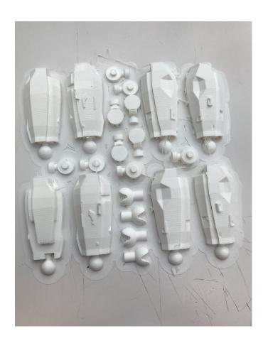
Eventually, after every part was printed correctly, all support material was removed, and everything was sanded smoothly, the Shell Walker was ready for assembly. Most parts were printed as two halves (to minimize support material). These halves were attached to each other with metal pins and plastic glue (the metal pins keep the parts in place while the glue is drying, while also providing extra solidity).
