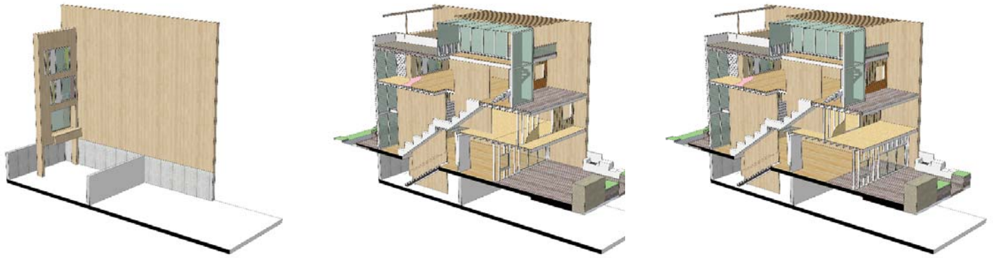
The structural system based on 2 fixed walls and infill allows for flexible back facade
