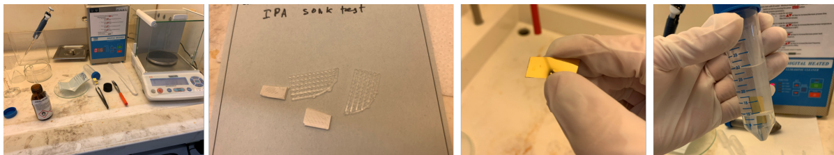
Figure A.2: Chemical exposure tests of 1M NH 3 (aq), 1M HCl(aq), IPA were performed on PLA and polypropylene printed parts.
