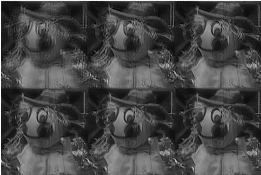
Figure B-5: Estimated object after 1, 5, 10, 15, 20 and 25 iterations. The algorithm used is: TIP3A, M = N = 15 , r_{\mathbb{X}} = 6 , w = 2000 , \epsilon = 10^{-4.4} . Images with isoplanatic aberrations are used as an input here.
