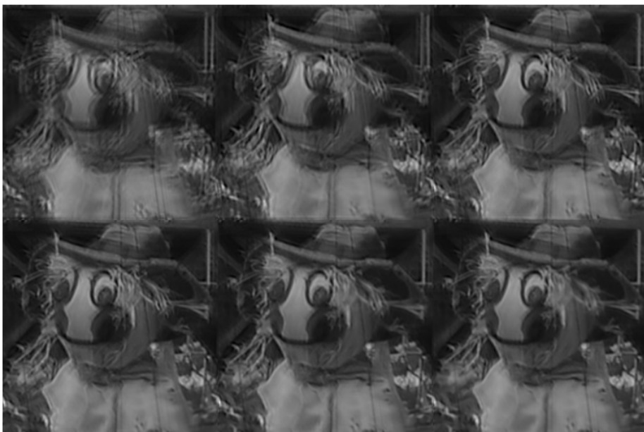
Figure B-4: Estimated object after 1, 5, 10, 15, 20 and 25 iterations. The algorithm used is: TIP3A, M = N = 7 , r_{\mathbb{X}} = 6 , w = 2000 , \epsilon = 10^{-4.4} . Images with isoplanatic aberrations are used as an input here.
