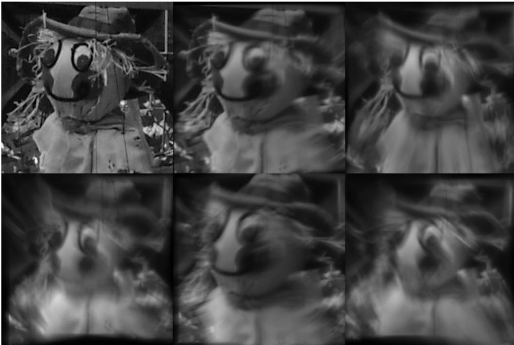
Figure 3-3: The object in the first sub-figure is deteriorated by different space-variant point spread functions and with the addition of white Gaussian noise with standard deviation, \sigma = 10^{-3} . Space-variant point spread functions are calculated in a simulation with a single phase screen in between the object plane and the pupil plane. Figure 2-3 shows how a phase screen models the induced phase aberration outside the pupil plane and how the aberration is projected onto the pupil plane. This allows the calculation of a point spread function that depends on the location of a point in the object. These space-variant point spread functions are used to deteriorate the object. The resulting images are shown in the other sub-figures.
