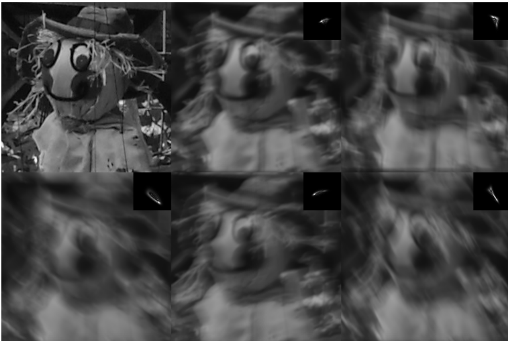
Figure 3-2: The object in the first sub-figure is deteriorated by different point spread function and with the addition of white Gaussian noise with standard deviation, \sigma = 10^{-3} . This deterioration is performed by convolution. Convolution can be calculated efficiently in the frequency domain. The resulting images are shown in the other sub-figures. The top right corner of the blurred images shows the corresponding point spread function.
