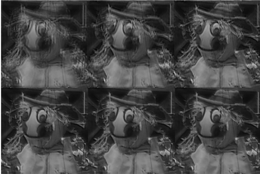
Figure B-1: Estimated object after 1, 5, 10, 15, 20 and 25 iterations. The algorithm used is: TIP, r_{\mathbb{X}} = 6 , \epsilon = 10^{-4.4} . Images with isoplanatic aberrations are used as an input here.
