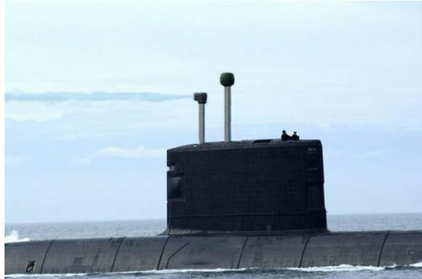
Figure 2.1: A submarine with a raised snorkel and exhaust mast (the left and right mast respectively) [84].
