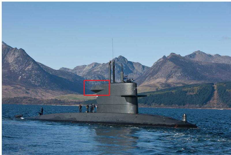
Figure 3.2: The sail of a Walrus class submarine, the location of the exhaust is indicated with the red box [53].
