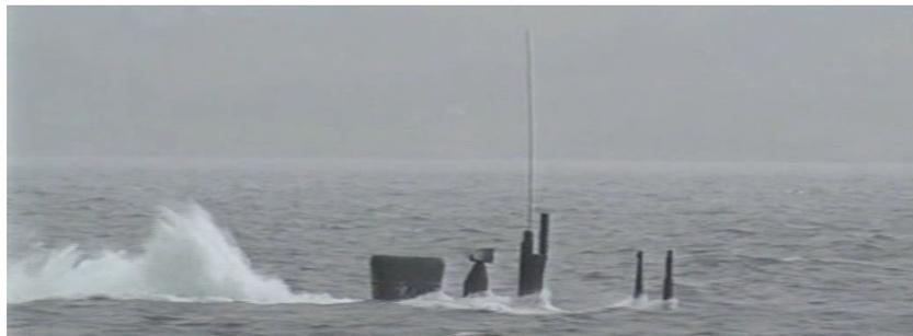
Figure 2.2: A submarine of the Walrus class sailing while using a snorkel. The visible masts on this image are, from left to right: the snorkel mast, the radar mast, the communications mast, the observation periscope and the attack periscope. On the left the surface elevation due to the submerged exhaust is visible [52].
