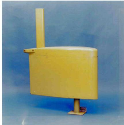
Figure 8.2: Photograph of the model used in the model tests by MARIN. In this photograph the adapted exhaust is fitted on the sail [79].
