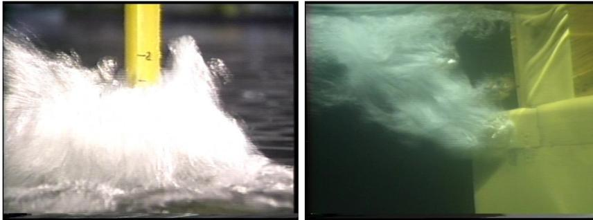
Figure 8.4: Surface and submerged photo,  $\phi_V = 1 \cdot 10^{-2} \text{ m}^3/\text{s}$  [79].
