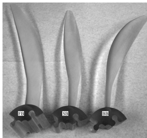
Figure 1.6: Forward-swept blade (FB), straight blade (SB) and backward-swept blade (BB) used for experimental investigation [5].
