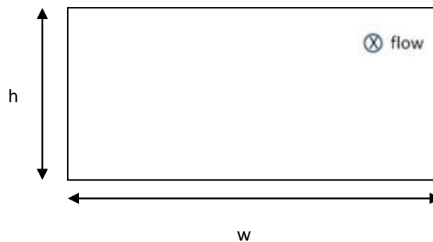
Figure 2.1- The cross section of single micro-channel
