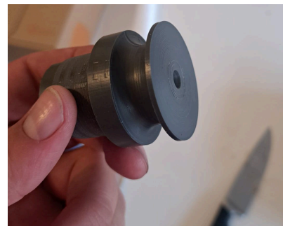
Figure 5.3k: Diabolo wheel made on the lathe.
