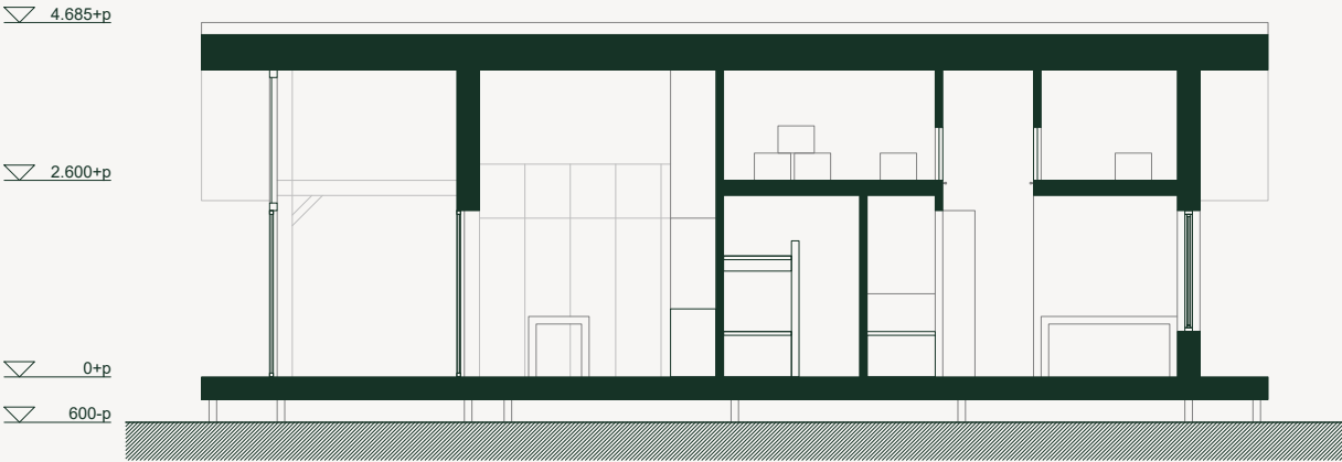
Figure 32: Section housing type Starling (Own work)
