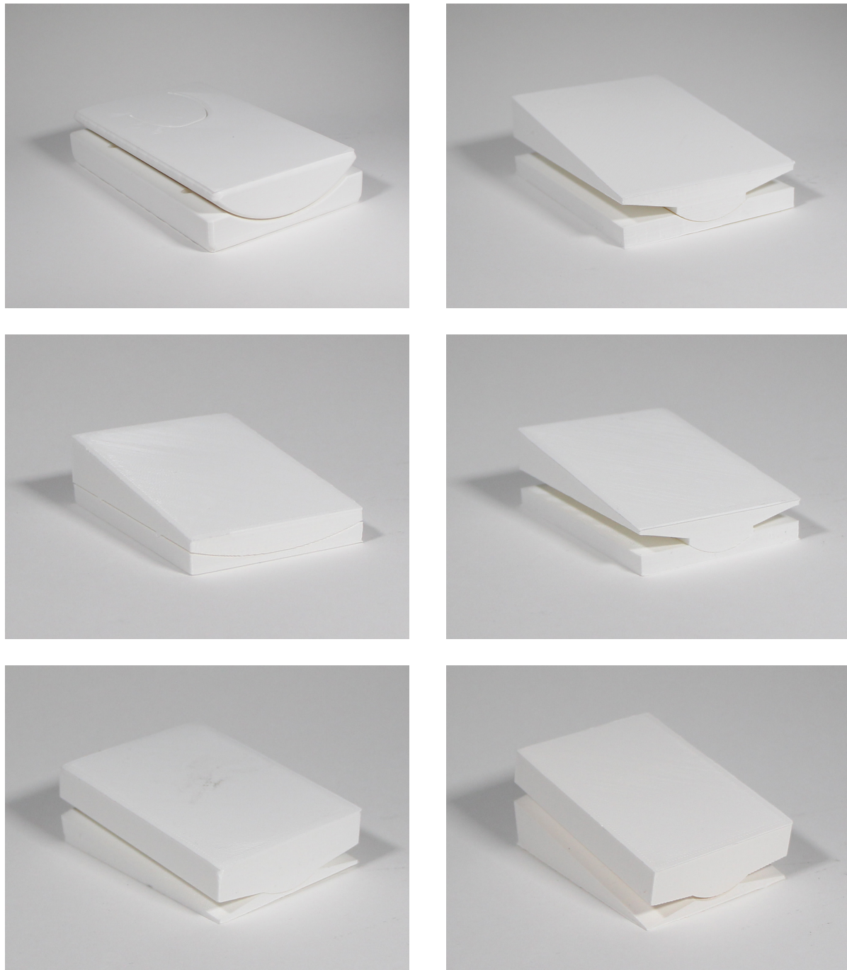
Figure 64. Iterations on the two-part bottom design, chronologically ordered from top left to bottom right
