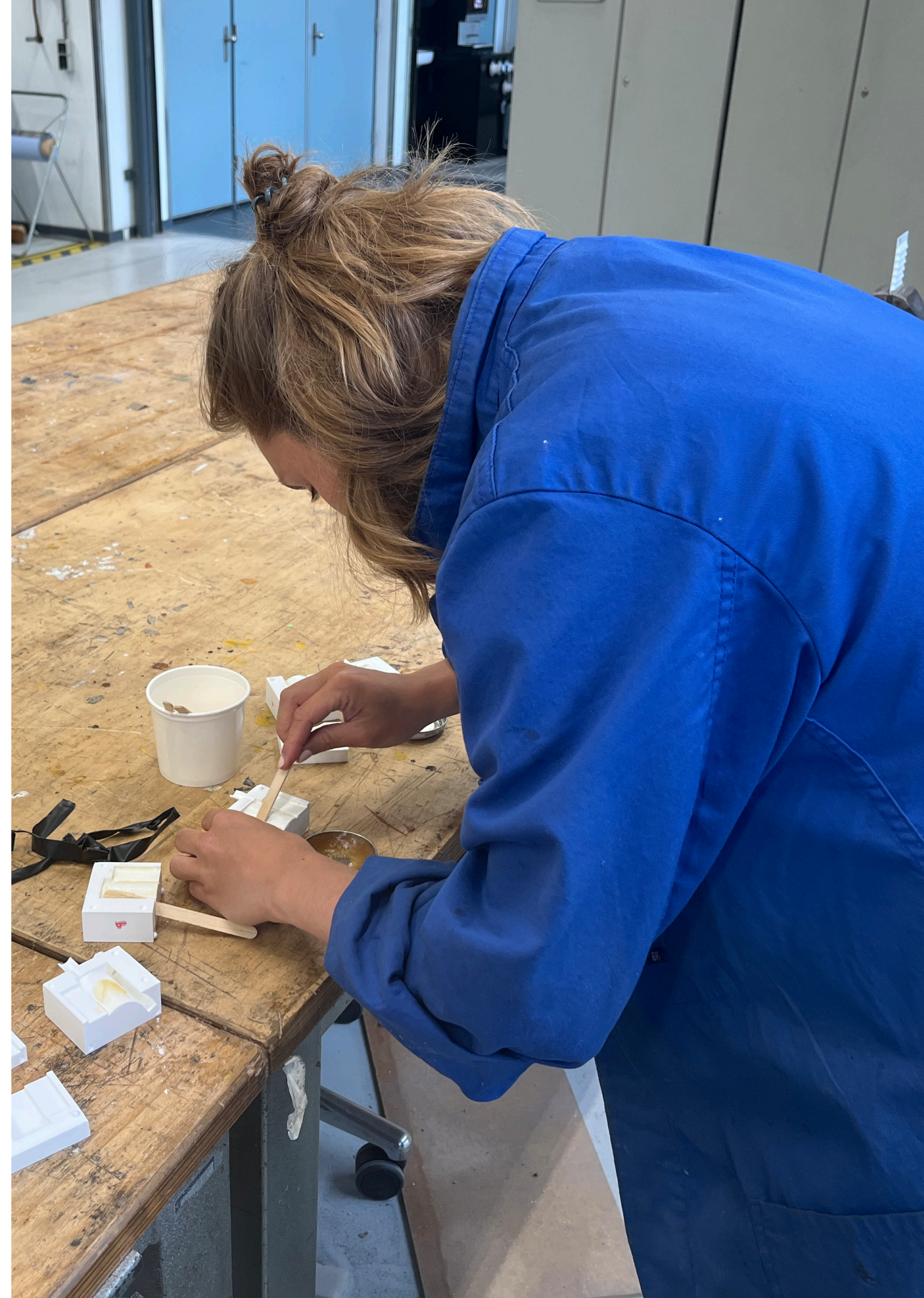
Figure 94. Preparing 3D printed molds for silicon pouring
