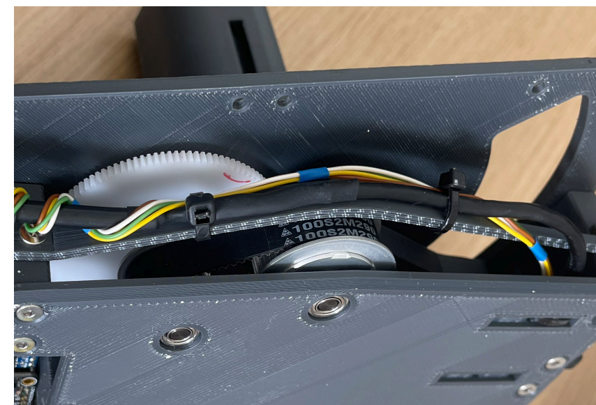
Figure 31. Shell movement gears, top view
