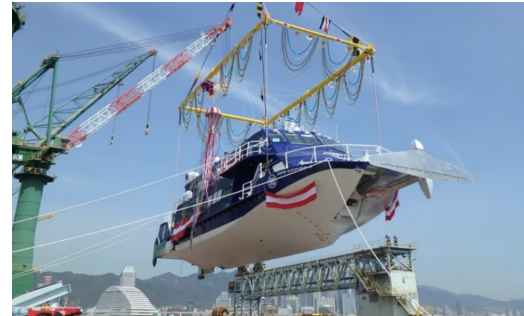
(b) Retracted hydrofoils (Baird Maritime, 2020)
