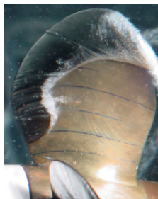
(b) Transcavitating Newton-Rader series derived propeller (Gaggero & Brizzolara, 2009)
