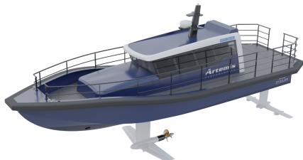
(a) The non-retractable (tandem configuration) work boat EF12
