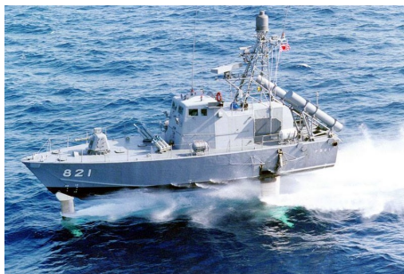
(a) High-speed foiling with extended foils (Asian Military Defense Review, 2013)
