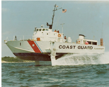
(a) High-speed foiling with extended foils (US Coast Guard, n.d.)
