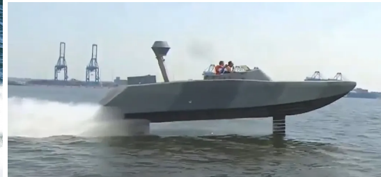
(b) Hydrofoil conversion of the Mk Mod 2 High Speed Assault Craft (Trevithick, 2019)
