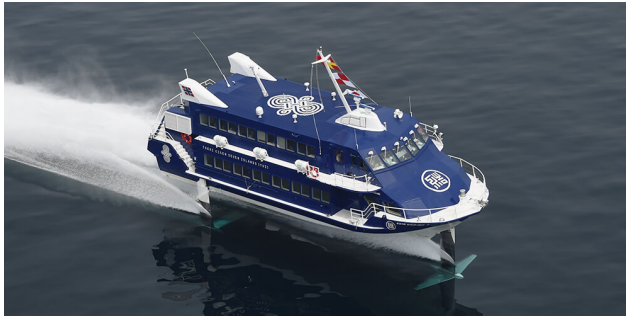
(a) Foiling at high speed with extended hydrofoils (Tokai Kisen, 2024)
