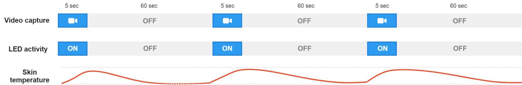
Figure 64: Proposed intervals of video capture. The red line represents the temperature change of the skin, which should be insignificant.
