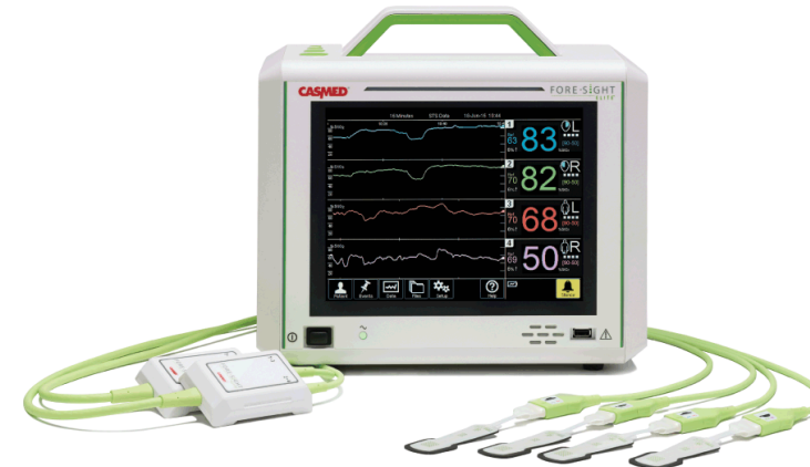
Figure 28: Near-infrared spectroscopy device containing the main monitor unit and four probes 48 .
