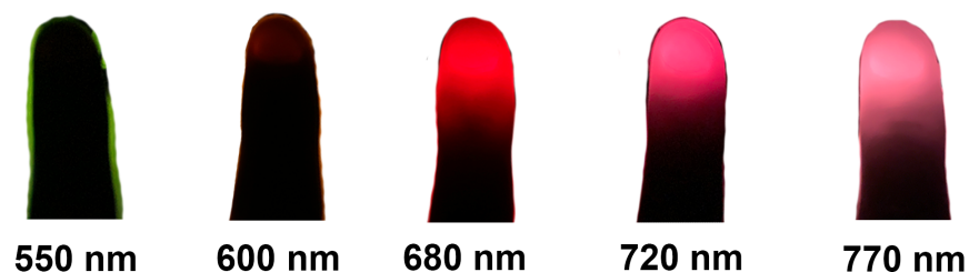
Figure 61: Fingertips illuminated by LEDs with different wavelengths to see how much is passed through the tissue. Wavelengths above 800 nm were not picked up by the smartphone camera as it has an infrared filter. The longer wavelengths showed significantly better light transmission.
