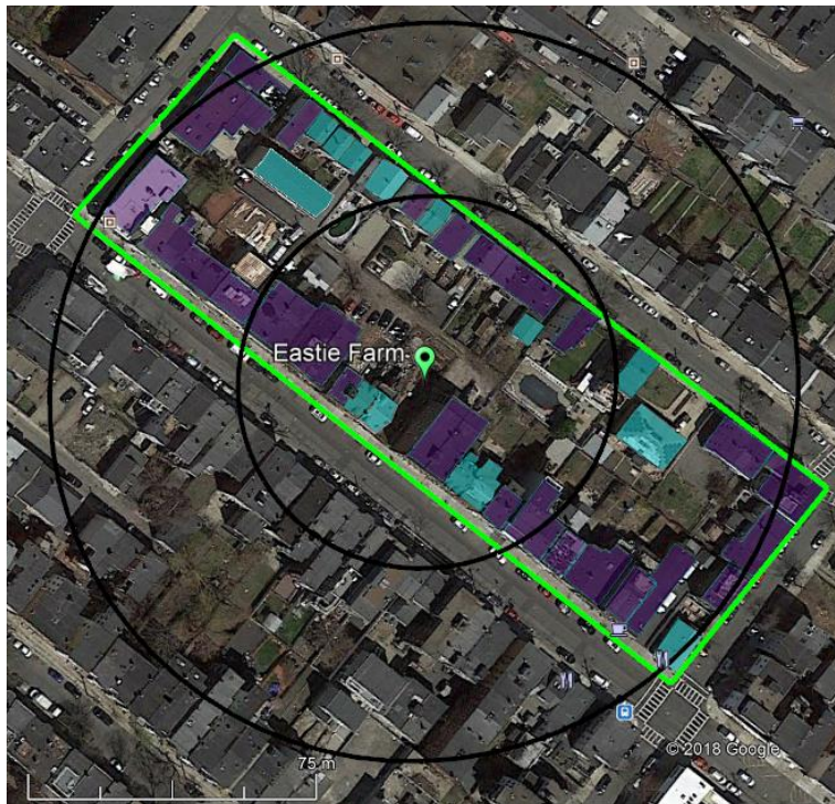
Figure 34 Flat (purple) and pitched (turquoise) roof surfaces within a 50-meter radius (inner circle) and a 100-meter radius around the farm and within Eastie Farm's housing block.
