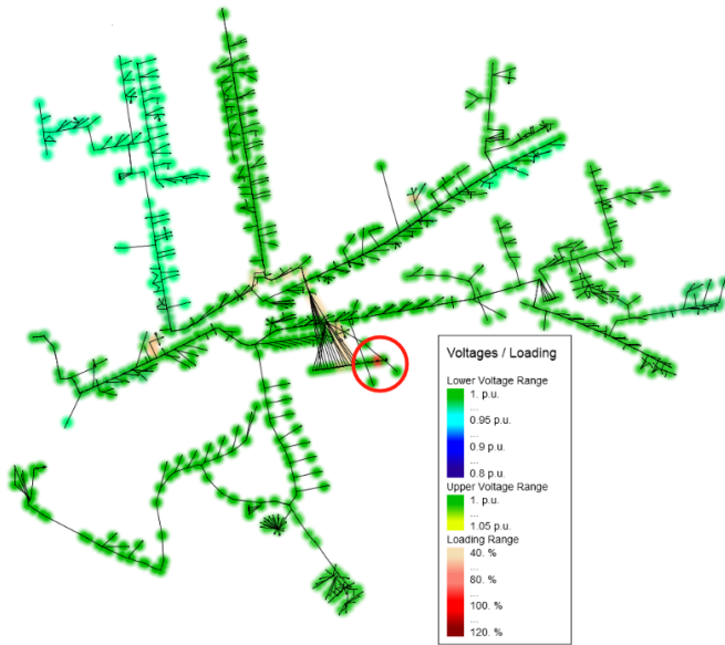
Fig. 4: Heat map showing the under-voltage region in the urban grid with 80% EV penetration.
