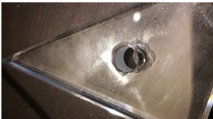
hole in glass, drilled from just one side->fractured (own image)
