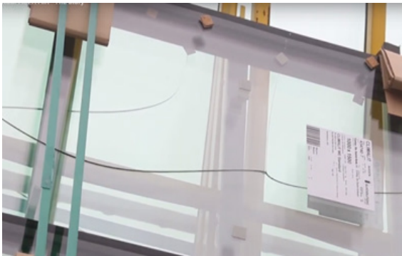
Figure 3.1.2.5 Corks will be placed on top of the glass pane for it to transfer (AGC)
