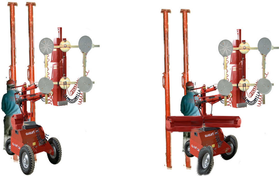
Figure 5.3.3.4 :Glasslift working order based on http://www.glgcan.com/ (width= 618 mm to drive through hallways).
