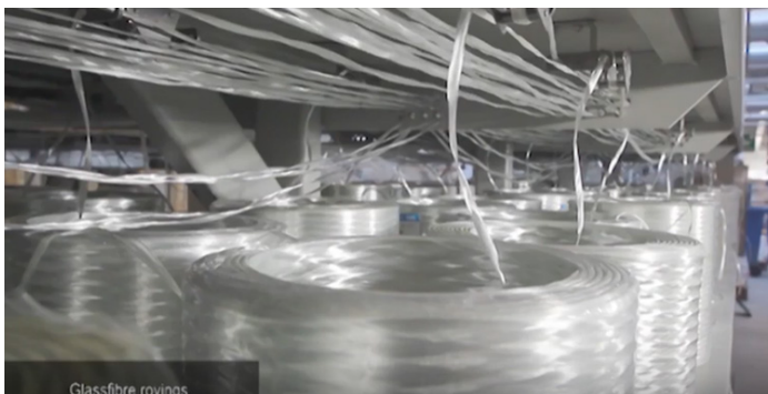
Figure 5.7.1.1: Pultrusion process of GRP at fiberline .
