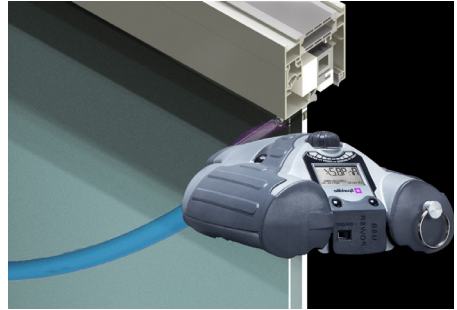
Figure A.4.2: Argon measuring device to measure will be applied at the top of the window.
