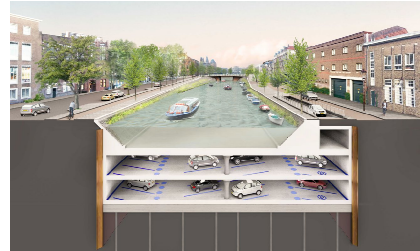
34 Subcanal parking can provide ample parking space without taking up any surface space.
