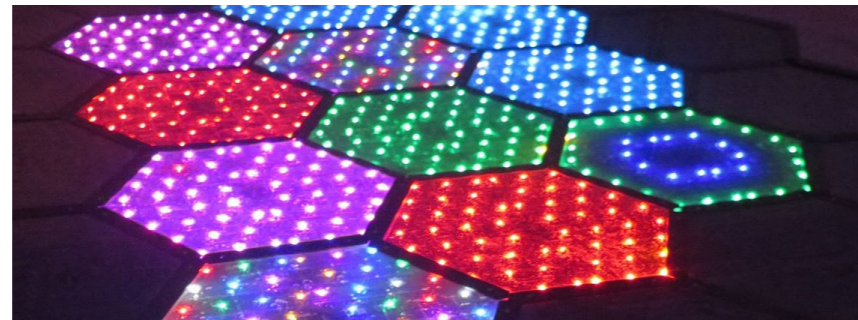
52 Solar Roadways pilot installation of a digital road surface that can be updated in real-time.
