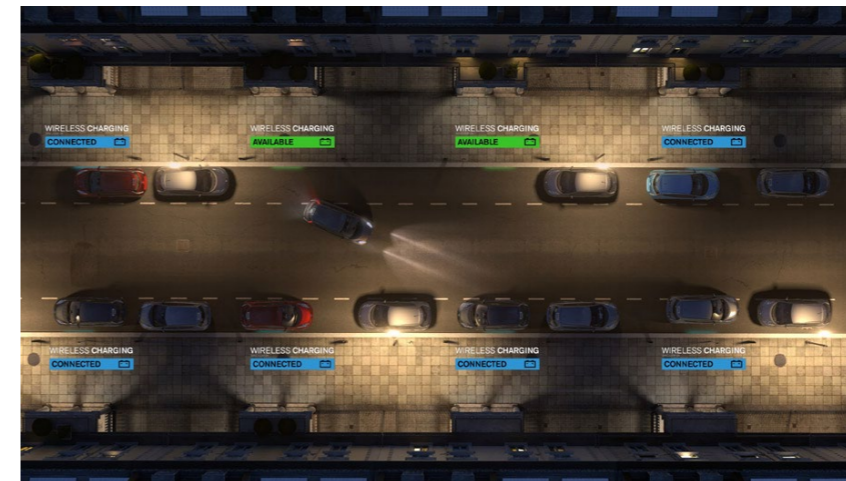
51 Concept for wireless charging through a road surface by Foster + Partners and Nissan.
