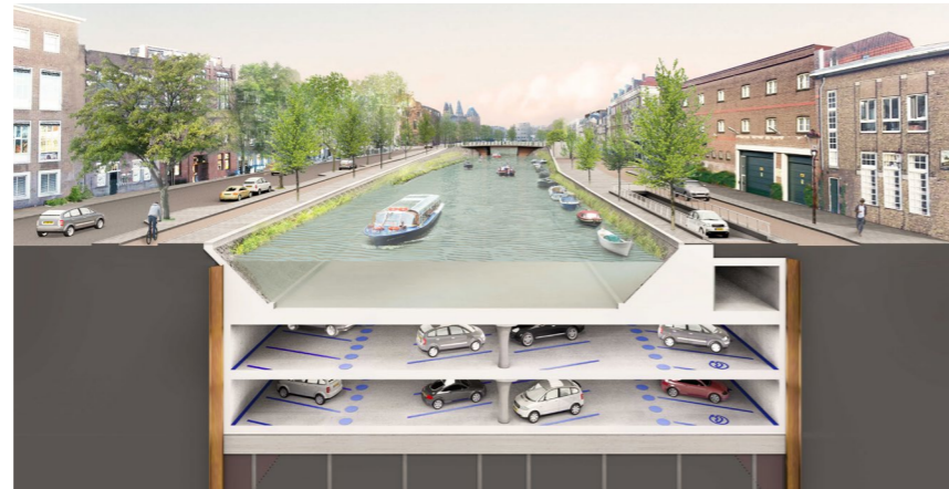
60 Planned parking garage under the Boerenwetering canal.
