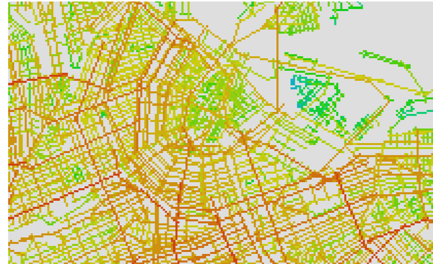
107 Fractional Mean Depth Space Syntax of Amsterdam city centre showing the central position of radial streets in the network. The red and orange lines denote that streets are well-connected streets while the yellow to green lines indicate that streets are more secluded within the network.
