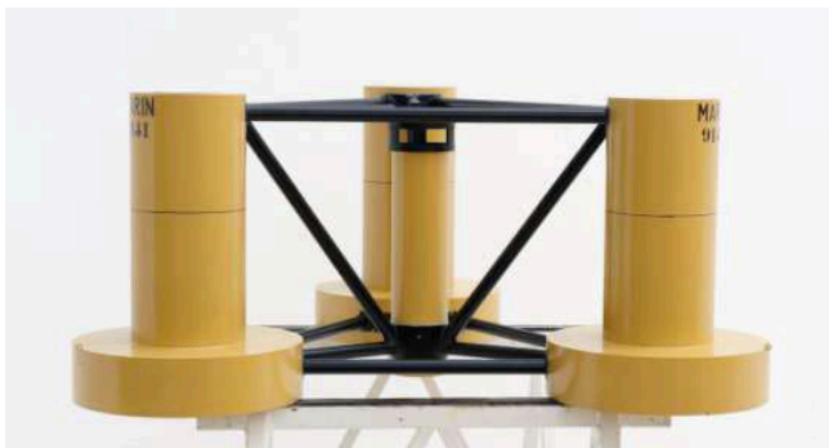
Figure 3.1: 1/50 model scale OC4 floater [33]
