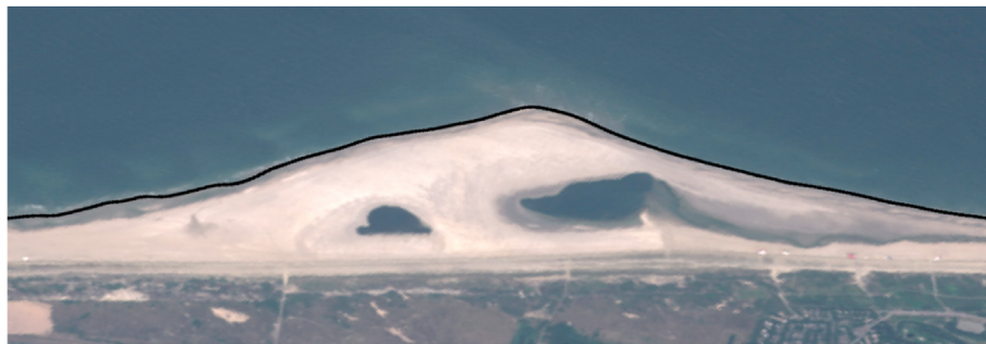
Fig. 4. Satellite image acquired by the Sentinel 2 satellite acquired on 12-03-2015 10:33:27 (GMT) for the Sand Motor study site. The derived SDS is plotted in black.
