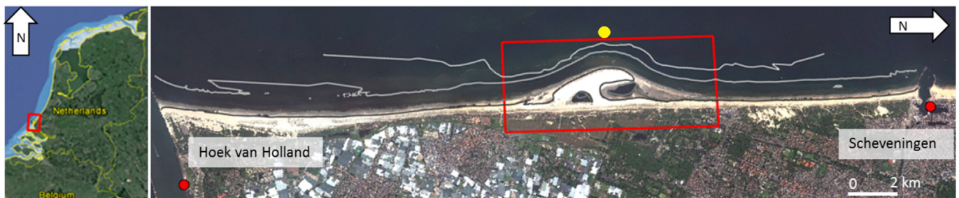
Fig. 1. Overview of the Dutch Delfland coastal cell bordered by Hoek van Holland (left) and Scheveningen (right). The Sand Motor study site is indicated in red. Depths at the -8 m, -5 m and +2 m NAP iso-contours are indicated in grey. The underlying satellite image (SPOT mission) was acquired on 18-05-2014. The water level measurement stations of Hoek van Holland and Scheveningen are indicated by means of a red dot. A nearshore location at the -10 m NAP depth contour, on which nearshore wave data are available, is indicated in yellow. (For interpretation of the references to colour in this figure legend, the reader is referred to the Web version of this article.)
