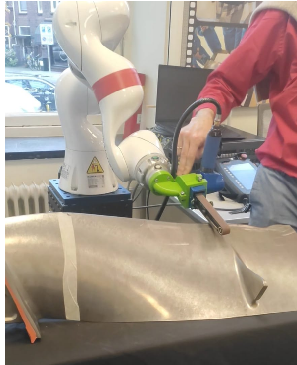
Fig. 1: A representative example of collaborative blending during jet engine turbine blade maintenance, where the developed interface can replace the existing tools (green). This use case is part of the BrightSky project.
