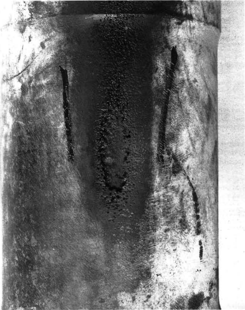
Figure 5.8.3. Cavitation corrosion in diesel engine cylinder liner on the cooling water side.
