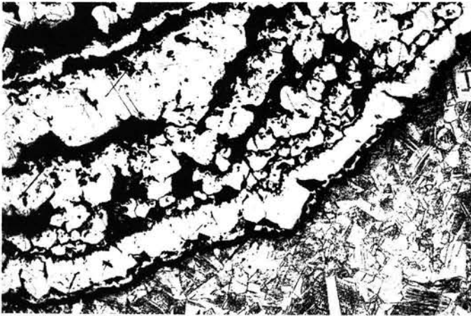
Figure 5.5.2. Plug type dezincification. a. schematic cross section; b. photograph of tube with plug type dezincification; c. photomicrograph of boundary between porous copper residue (upper left) and unattacked brass.
