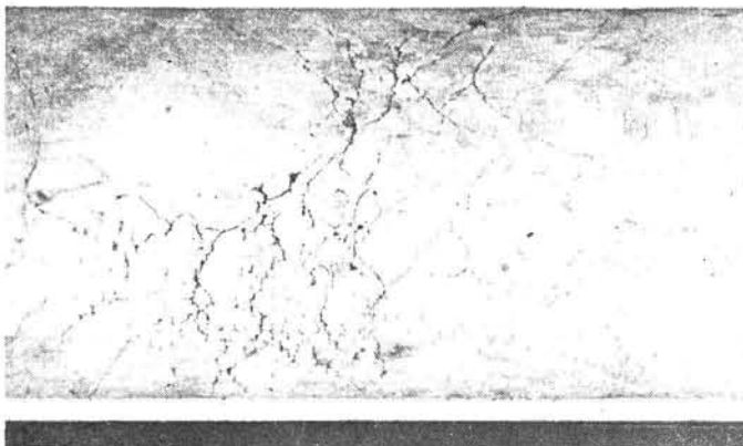
Figure 5.7.3. Stress corrosion cracking of a tube from a citric acid evaporator. Material: stainless steel type AISI 316.
