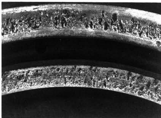
Figure 5.9.1. Fretting corrosion of thrust rings.
