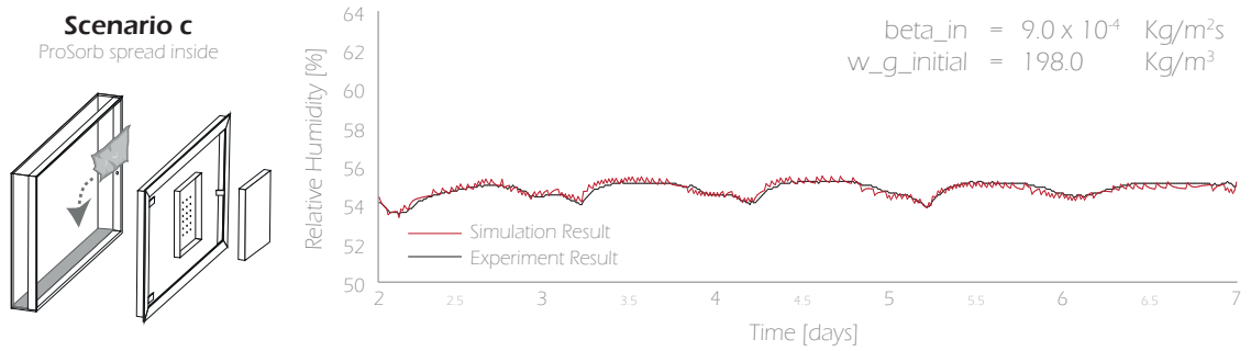
Figure 51: Least square fit analysis: Scenario c - With AER = 1.33 ac/d
