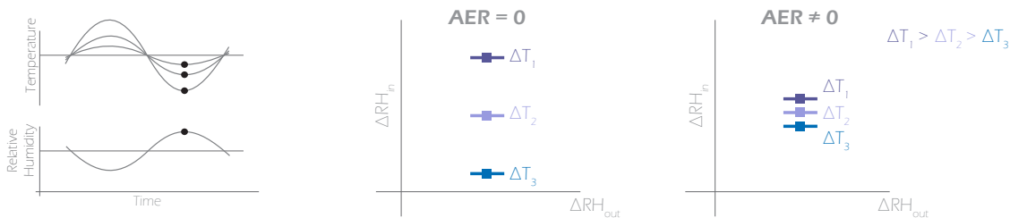
Figure 87: Analysis of the sensitivity trends when \Delta RH_{out} is fixed and the \Delta T is free
