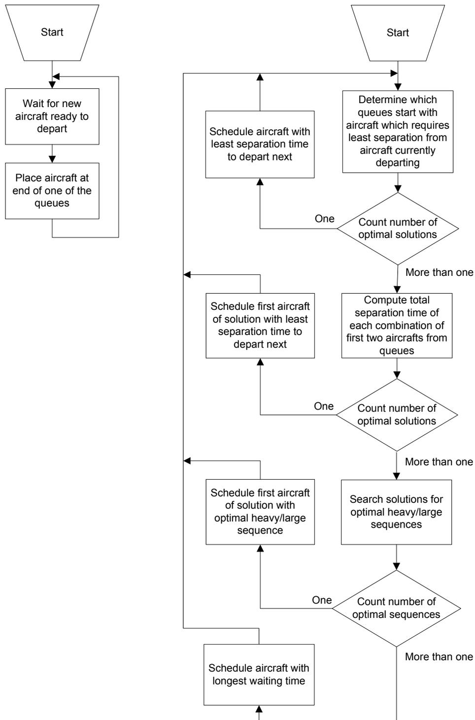
Figure 3.3: Flow diagram of a greedy search algorithm
