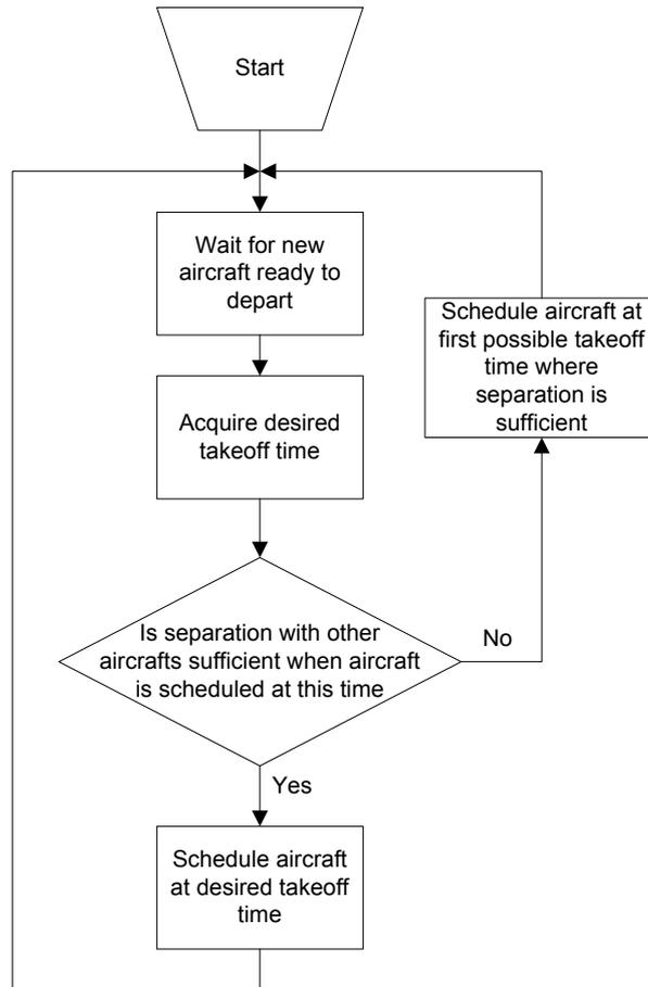
Figure 3.1: Flow diagram of a first come first served algorithm
