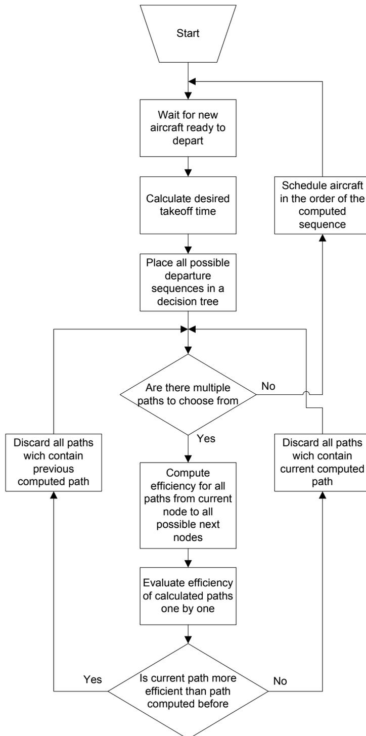
Figure 3.2: Flow diagram of a branch and bound algorithm
