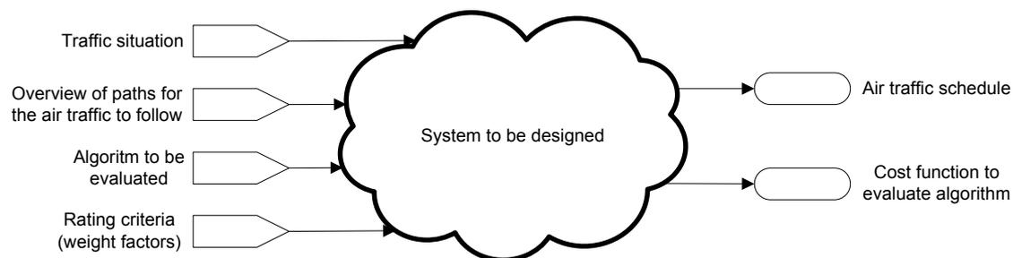
**Figure 2.16: Functional overview of the system to be designed**
