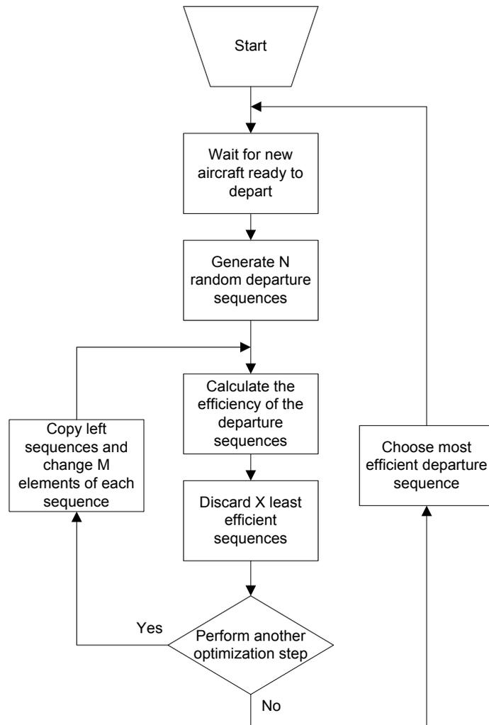
Figure 3.4: Flow diagram of a genetic algorithm
