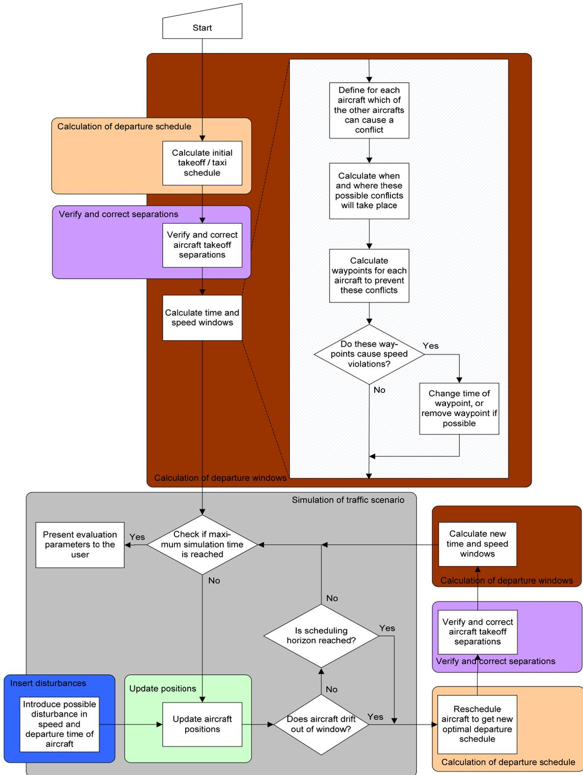
Figure 4.4: More detailed functional overview of the system to be designed
