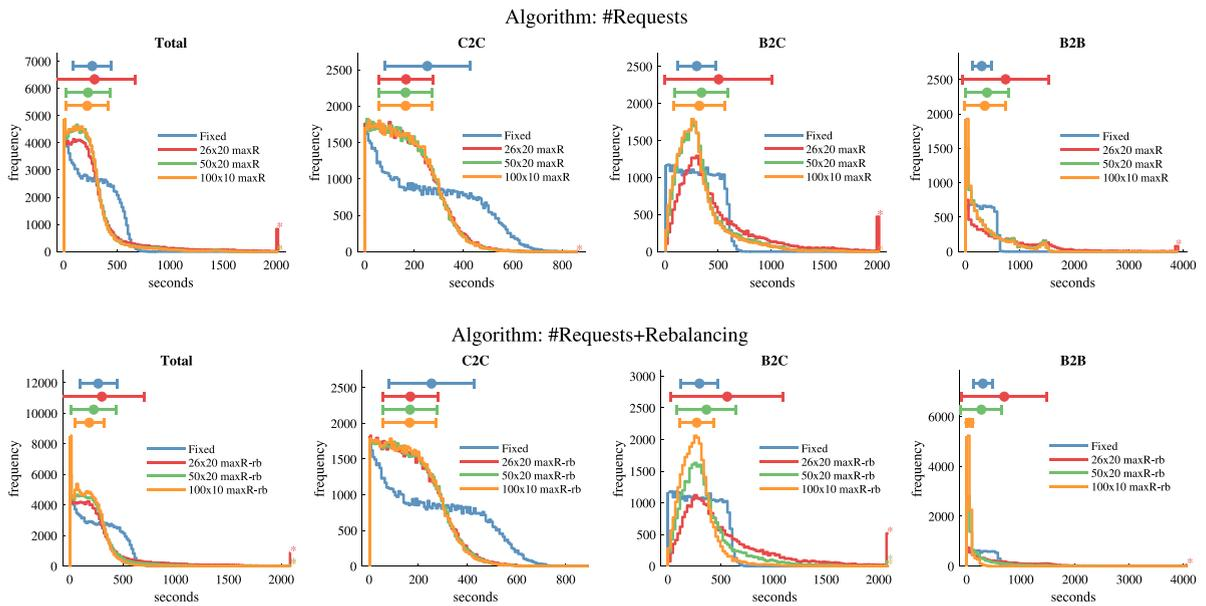
**Fig. 11.** Passenger total waiting time distributions with and without rebalancing for passenger groups (Total, Corridor-to-Corridor, Branch-to-Corridor, and Branch-to-Branch), for all tested scenarios. Bars above each histogram display the mean and  $\pm 1$  standard deviation of each distribution. (For interpretation of the references to color in this figure legend, the reader is referred to the web version of this article.)
