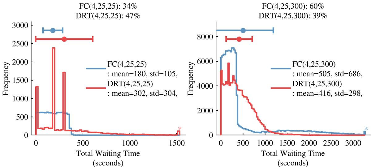
Fig. 10. Passenger total waiting time distributions for FC(4,25) (blue) and DRT(4,25) for the lowest (left) and highest (right) demand levels. Bars above each histogram display the mean and  $\pm 1$  standard deviation of each distribution. (For interpretation of the references to color in this figure legend, the reader is referred to the web version of this article.)
