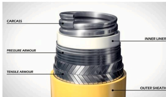
Fig. 1. Typical configuration of a flexible riser [3].
