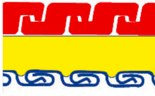
Fig. 2. Extrusion of the liner into the adjacent interlocked carcass [12].
