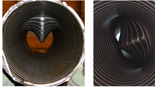
Fig. 3. “Heart” mode (left) [16] and “Eight” mode (right) [17].
