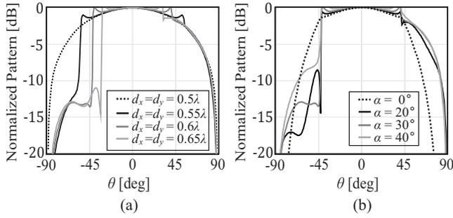
Fig. 2. Normalized active element pattern for an infinite array of stacked dipoles (a) with a tilted  $30^\circ$  varying the spacing between elements  $d_x$  and  $d_y$  and (b) with a periodicity of  $d_x = d_y = 0.6\lambda_0$  varying the inclination angle of the elements  $\alpha$ .
