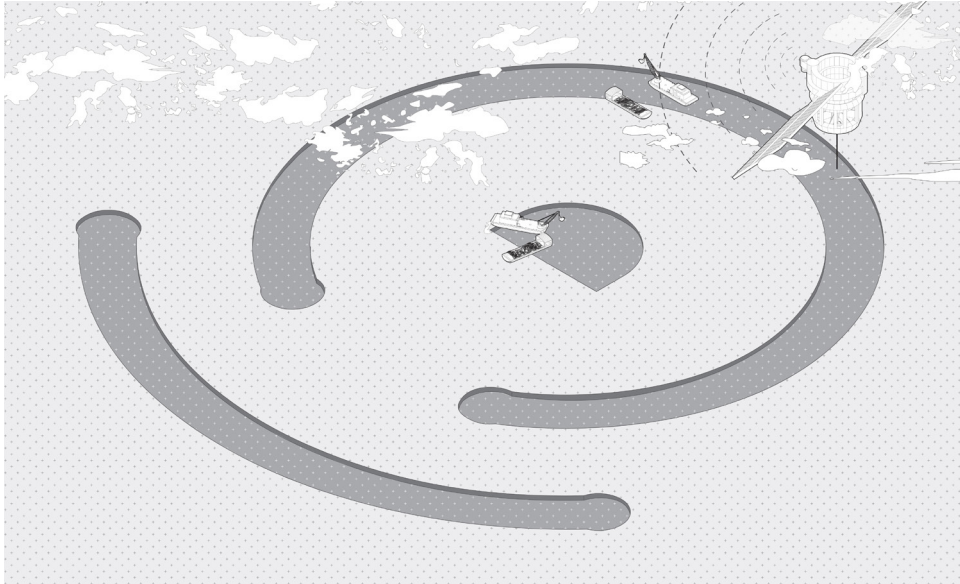
Step 1 - Removal of old sand using GPS
