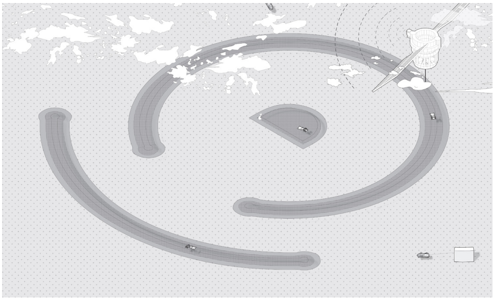
Step 4 - The rock foundation is "flattened" using robots guided by GPS
