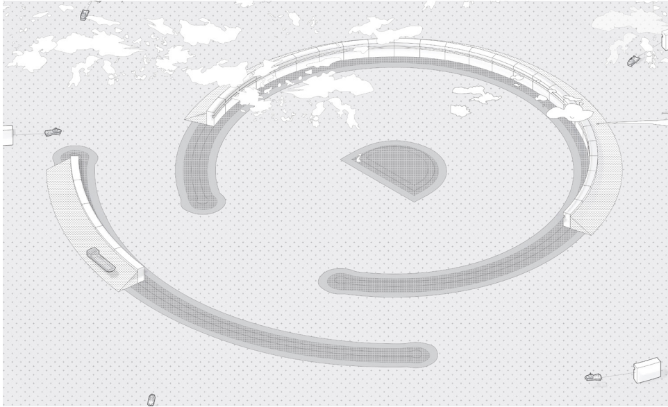
Step 5 - The Harbour, caisson box are arranged and recycled concrete protection ring is assembled
