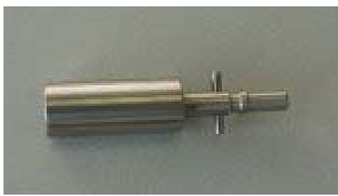
Fig.1A The stainless-steel head for a fuel pin.
