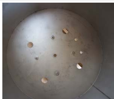
Fig.6 The bottom of the steel vessel. The four large holes will be used to insert spotlights, the central hole to insert the source tube and the two others to fill and drain the vessel.
