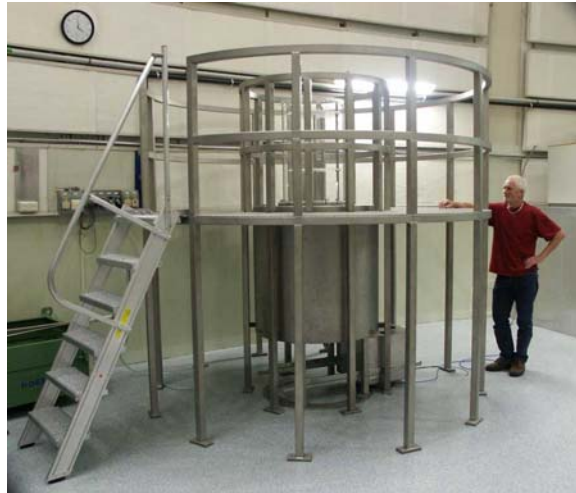
Fig.8 The main parts of DELPHI assembled together. Inside the loading platform, the steel vessel is mounted below which the drawer mechanism and the shielding box are seen. On top of the steel vessel, the acrylic vessel is mounted. Because of its transparency, this vessel is less visible.
