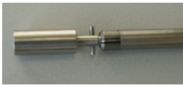
Fig.1B The stainless-steel head grabbed by the special handling tool.
