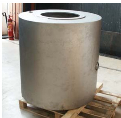
Fig.5 The stainless-steel vessel of DELPHI. The small flange on top of it will be used to mount two floats to control the water level inside.
