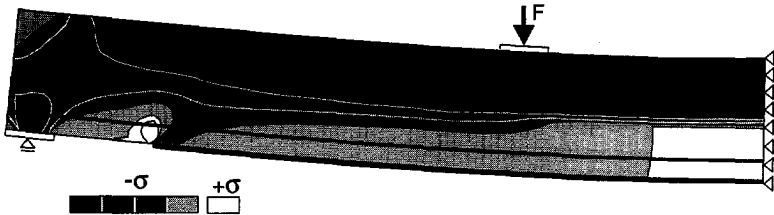
Fig. 10.1 Minimum principal stresses in finite-element model for a beam with a bonded-on plate stopped 200 mm short of the support
