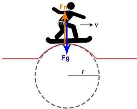
Figure 6: Model of a sit-snowboarder passing a hill
