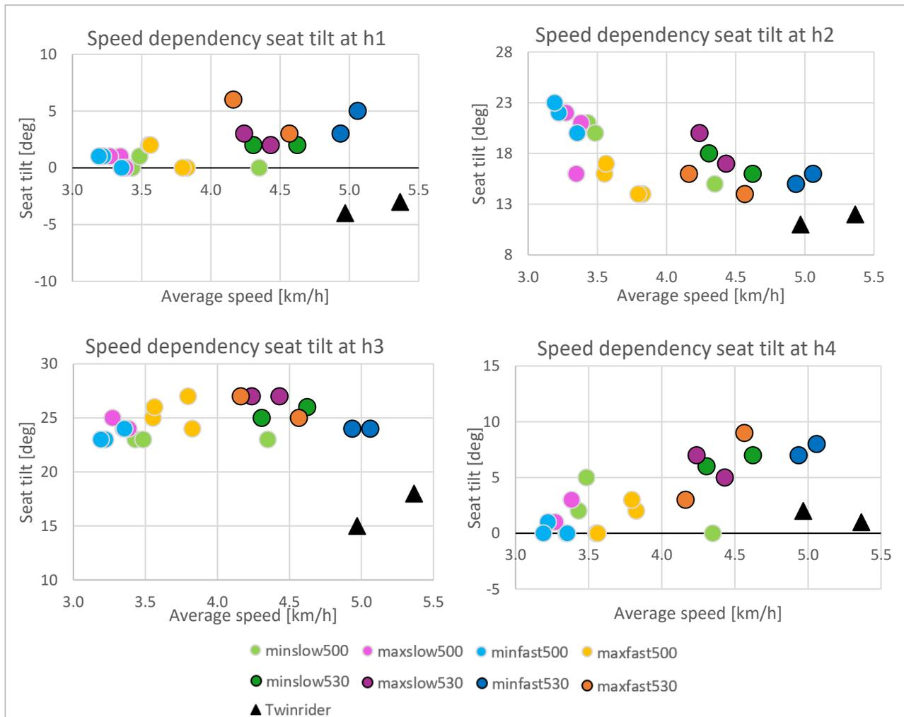
Figure 28: Seat tilt plotted against the speed for measuring locations 1 to 4 at the hill.
