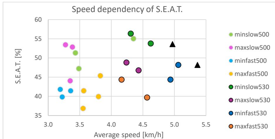
Figure 27: S.E.A.T. values plotted against riding speed for each run.
