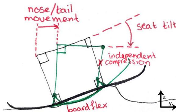
Figure 11: Schematic drawing of the functionalities of the Snowcruiser. Twinrider is shown in black, Snowcruiser is shown in green.
