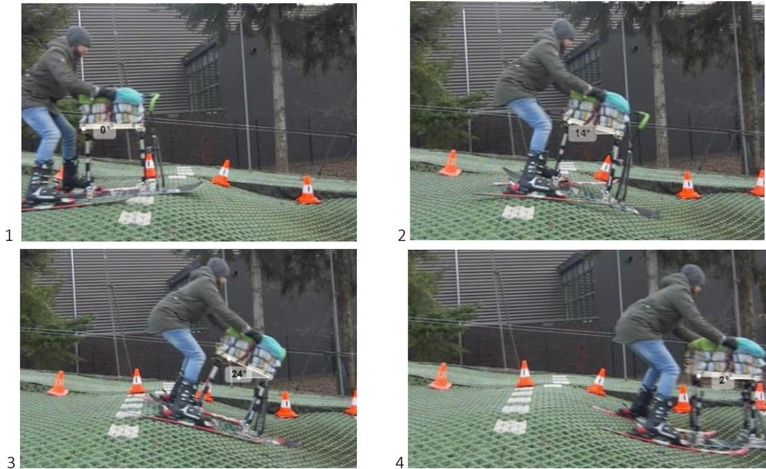
Figure 17: Measurement of seat tilt at 4 locations when passing the hill. Screenshots from 'maxfast500 run1'.
