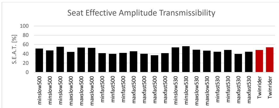
Figure 20: Seat Effective Amplitude Transmissibility values of all runs.
