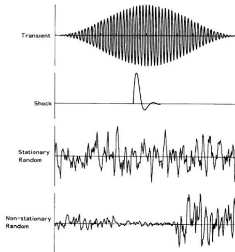
Figure 18: Examples of waveforms of different types of oscillatory motion. (Retrieved from Griffin, 1996)
