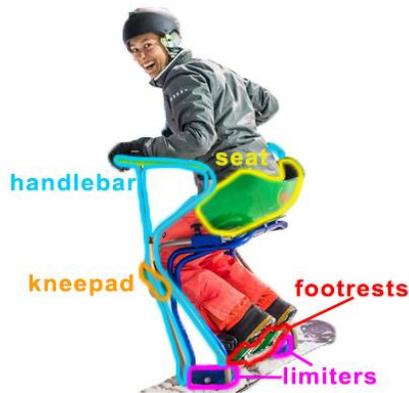
Figure 8: Elements included in the current Twinrider design
