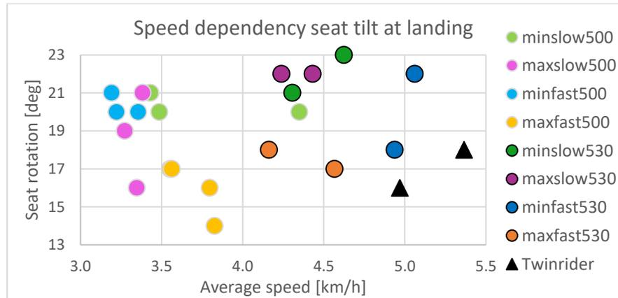
Figure 29: Seat tilt determined at the moment of landing after the hill is passed, plotted against speed.
