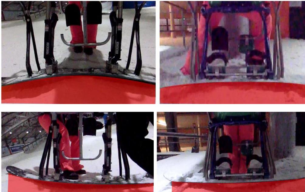
Figure 22: Board flexion is bigger for the Snowcruiser(left) than for the Twinrider (right).
