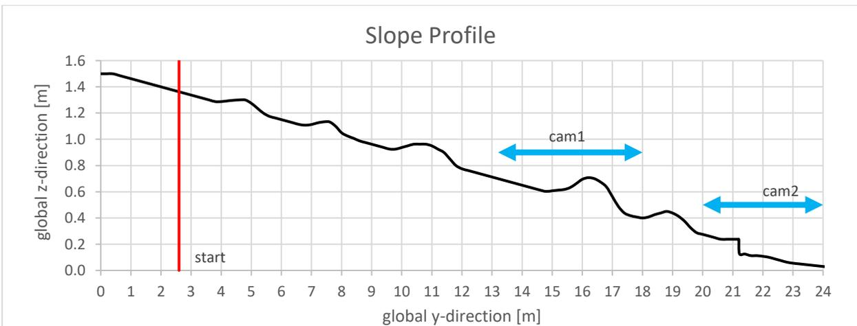
Figure 15: Section of the slope profile during the qualitative test.
