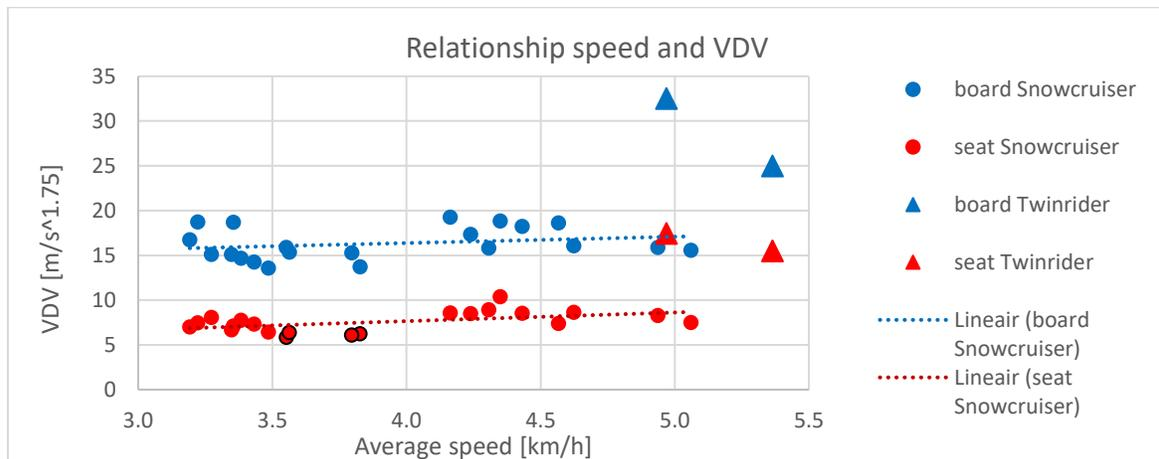
Figure 26: Vibration Dose Values plotted against riding speed for each run.
