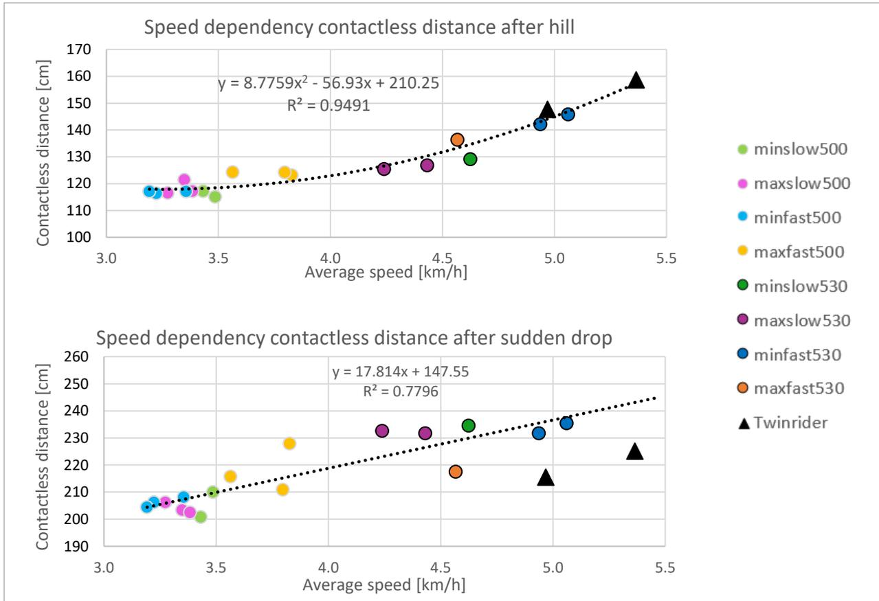
Figure 31: Contactless distances plotted against speed after passing the hill (top) and sudden drop (bottom.)
