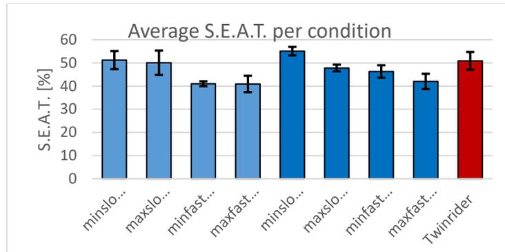
Figure 21: Seat Effective Amplitude Transmissibility averaged per condition.
