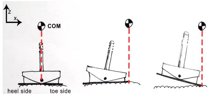
Figure 9: Working principle of the 'limiter'
