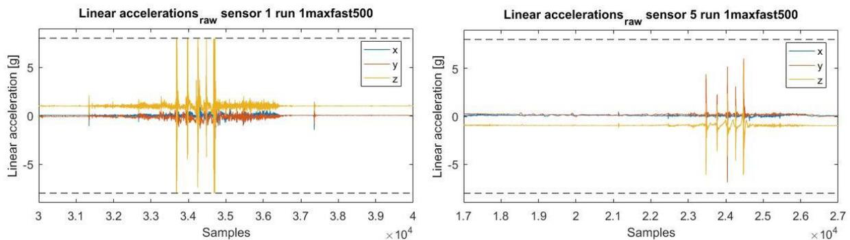
Figure 23: Raw linear accelerations of sensors 1 (left) and 5 (right) during a run with the Snowcruiser. In the left graph it can be seen that the sensor reaches the maxima of  $\pm 8g$ .
