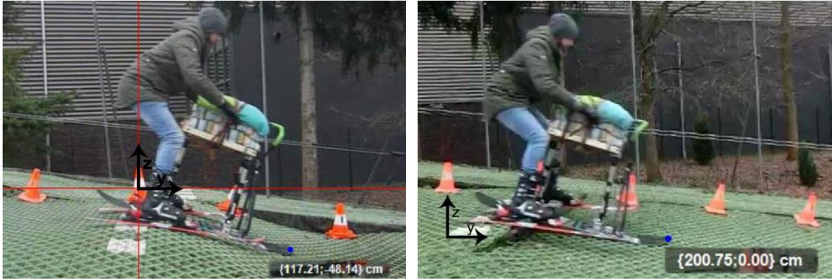
Figure 16: Measurement of contactless distances after hill (left) and sudden drop (right). Screenshots from 'minslow500 run 1'.
