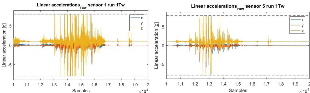
Figure 24: Raw linear accelerations of sensors 1 (left) and 5 (right) during a run with the Twinrider. Both sensors reach the maximum of  $\pm 8g$ .
