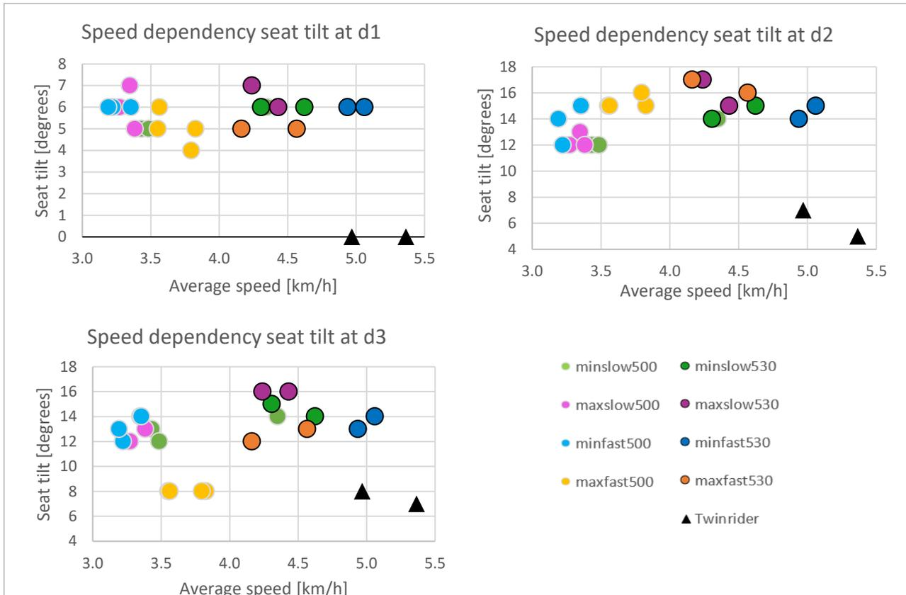
Figure 30: Seat tilt plotted against the speed for measuring locations 1 to 3 after the sudden drop.
