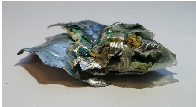
Figure 50: PCB in metal folded fragment
