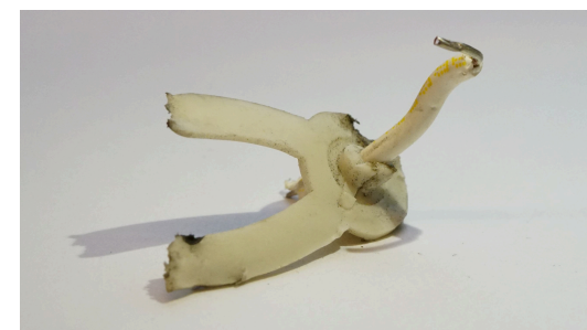
Figure 57: Wire remains in rubber grommet (Tubular)
