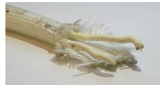
Figure 58: Wires remain in wire enclosure (Tubular)
