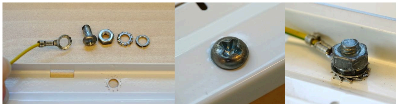
Figure 34: Use of O-rings, a nut, bolt and cable shoe on the reflector Sandwich
