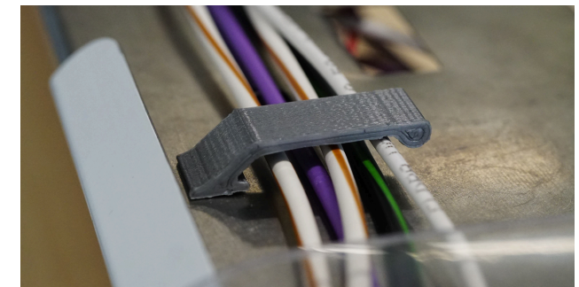
Figure 97: Guiding parts wires driver tray
