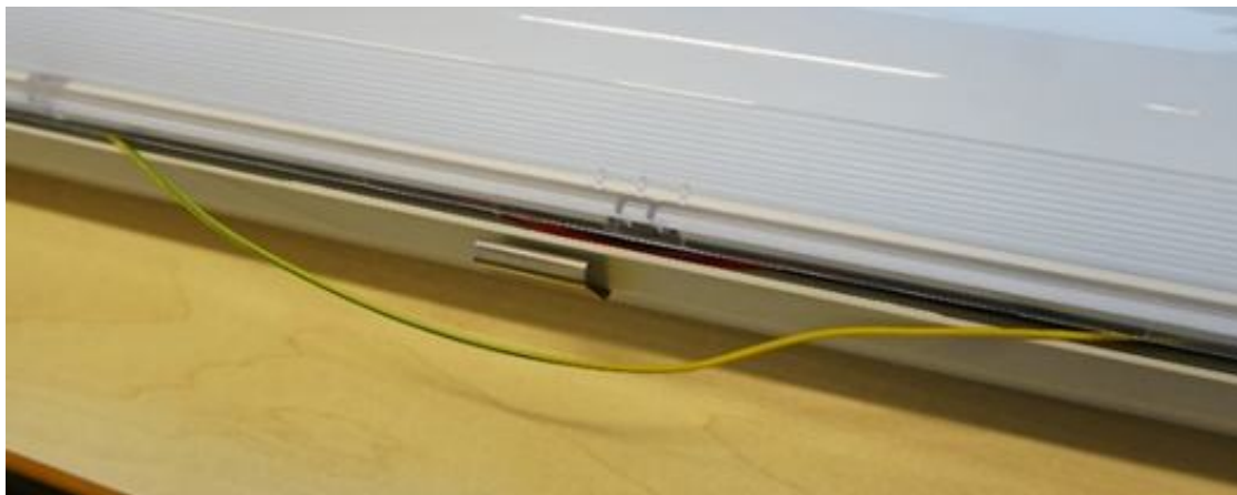
Figure 17: Wire in between the cover and housing Sandwich
