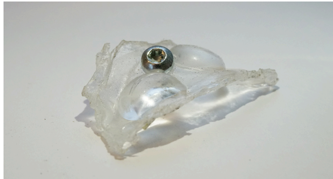
Figure 59: Screws remain in PC lens plates (Sandwich)
