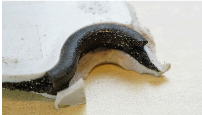
Figure 71: Glued silicone, note here it is not clamped in like the Sandwich. Most mixed fragments, namely 78% were like this
