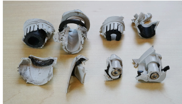
Figure L6: Fragments which will remain mixed when using a gasket (top 4 due to cable gland, left bottom 2 due to curvature end-cap, right bottom 2 due to screws)
