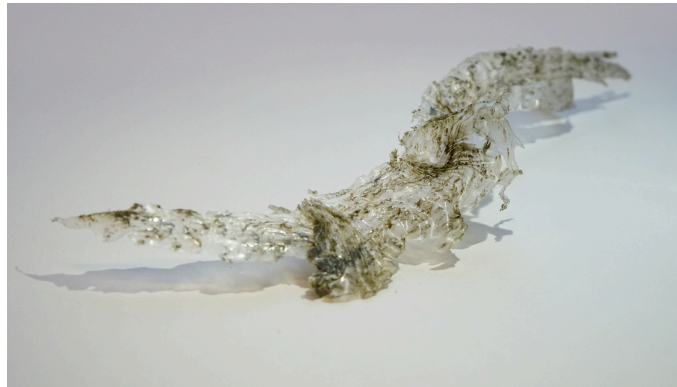
Figure 43: Flimsy PC, less than 0.5 mm thick
