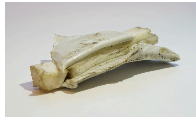
Figure 48: Clamped silicone in PC housing (Sandwich)
