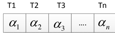
Figure 5.14: The individual chromosome representation in the genetic algorithm: \alpha is a float number ranging from 0 to 1
