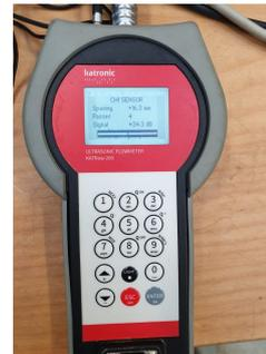
Figure 6.8: The control module of the flow meter
