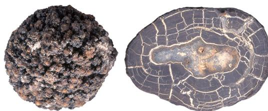
Figure 1.2: Outside and slice through of a manganese nodule [38].
