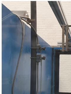
Figure 6.7: Attachment of the transducers to the PVC pipe
