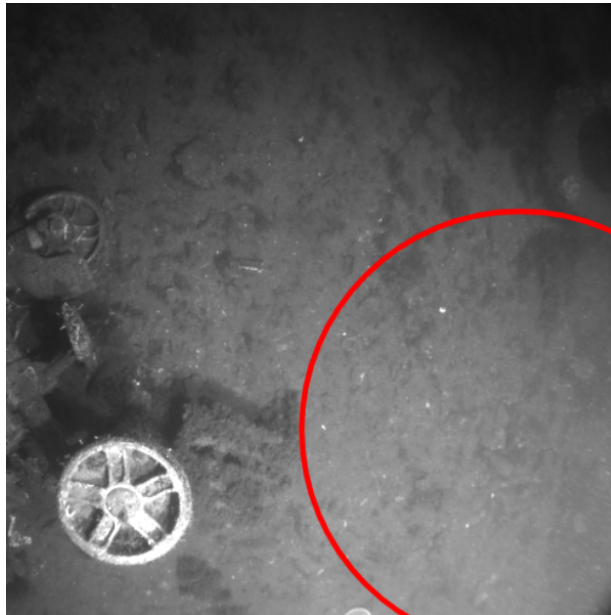
Figure 5.11: The red circle marks the area where the phenomenon of floating particles is more intense, in the Aqualoc dataset.
