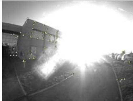
Figure 4.1: Light reflection causing loss in FOV. The small circles denote features that can be still extracted from the rest of the image. [72]
