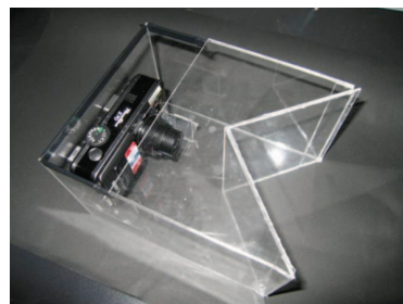
Figure 2.8: (a) Geometry and parameters of the refractive surface. (b) Camera housing that transforms monocular to a stereo system. The case is made of acrylic plates. (c) The obtained result when the camera with the case are placed into water.
