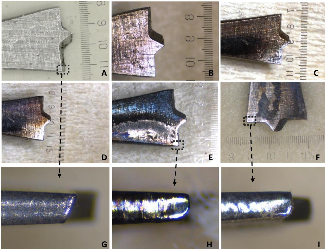
Figure 42 (A) Initial drill bit with burr visible, (B) after 5 drillings (C) after 50 drillings (D) after 90 drillings (E) after 90 drillings of 40 mm and 50 drillings of 60mm (F) after 90 drillings of 40mm, 60 drillings of 60mm and 5 drillings in bamboo (85mm), 10 drillings in wet Angelim de Campina (70mm) (G) side view of initial drill bit (H) side view of E (I) side view of F.
