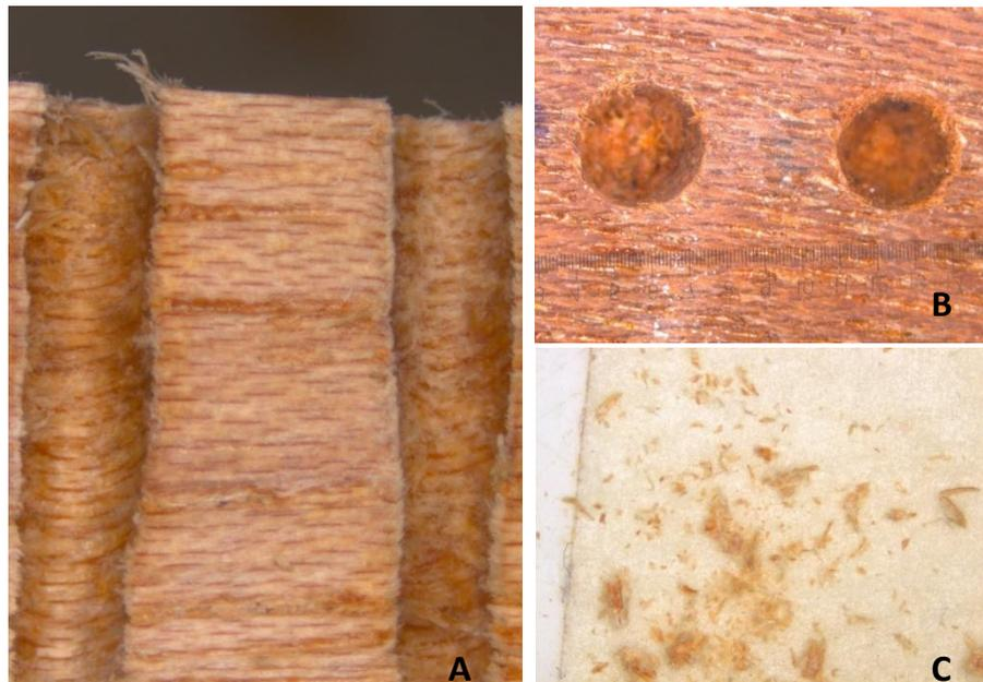
Figure 46 (A) Opened borehole with sawdust removed, sharp left and eroded right (B) Bore entry (sharp left eroded right) (C) Chips collected from borehole.
