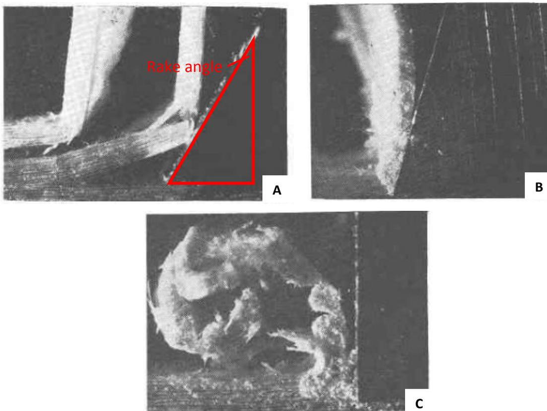
Figure 18 Different chip types: type 1 (A), type 2 (B), type 3 (C) the tool is in the right of the respective figures. The different chip types are obtained by changing the rake angle, approximately 35° at A to approximately 0° at C (Franz, 1955)
