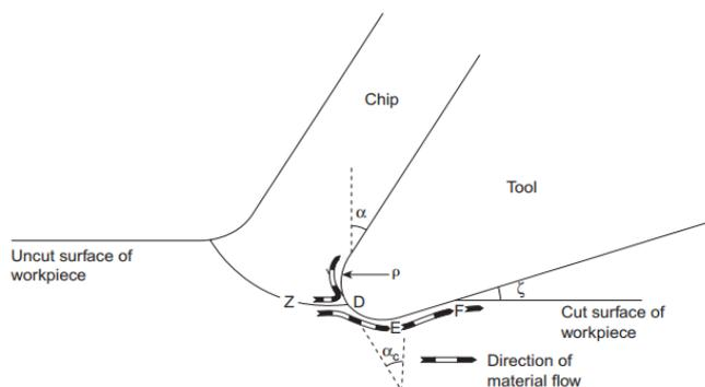
Figure 27 Clearance face rubbing Illustrated here for steel however also applicable for wood (Atkins, 2009).
