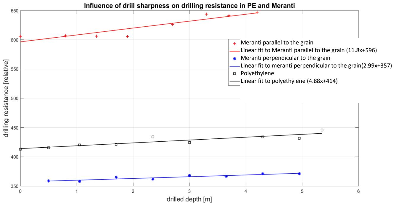
Figure 45 Influence of drill bit sharpness on the drill resistance in polyethylene and meranti (parallel and perpendicular to the grain).
