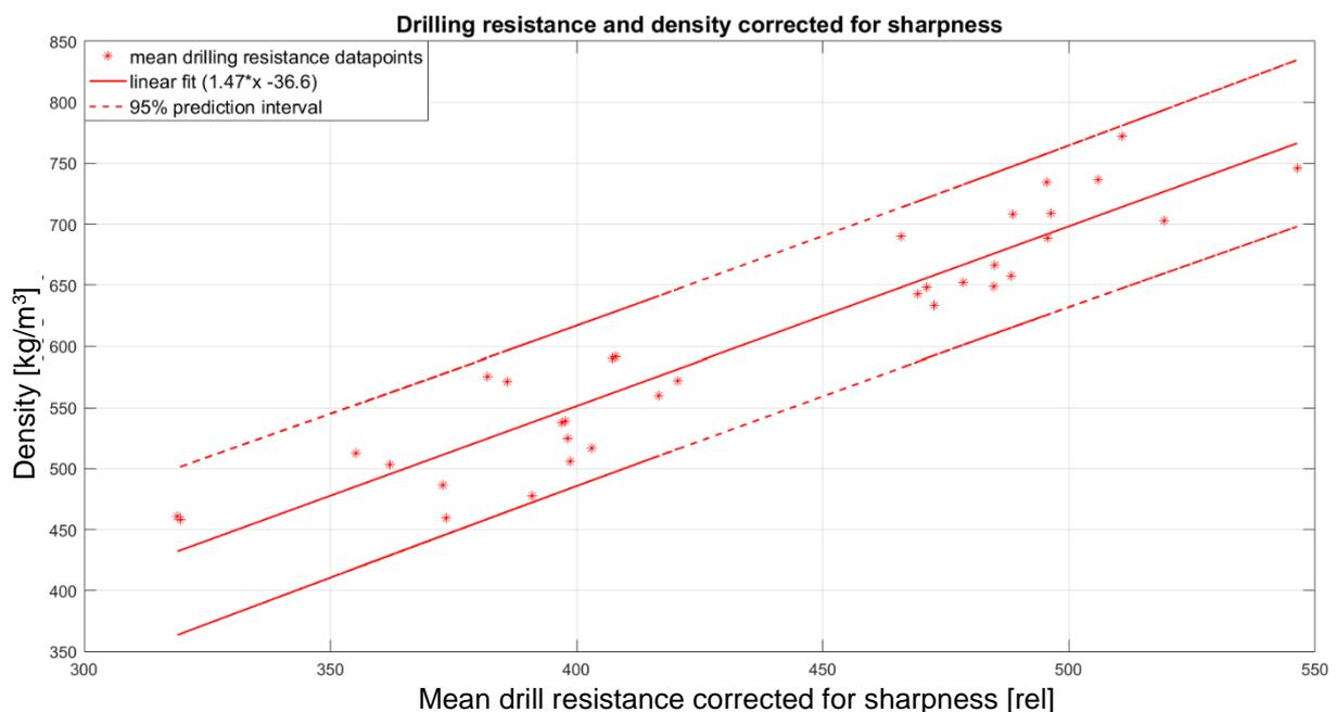
Figure 50 Mean drill resistance of conditioned meranti pieces corrected for sharpness versus density. The red line is the linear regression line.
