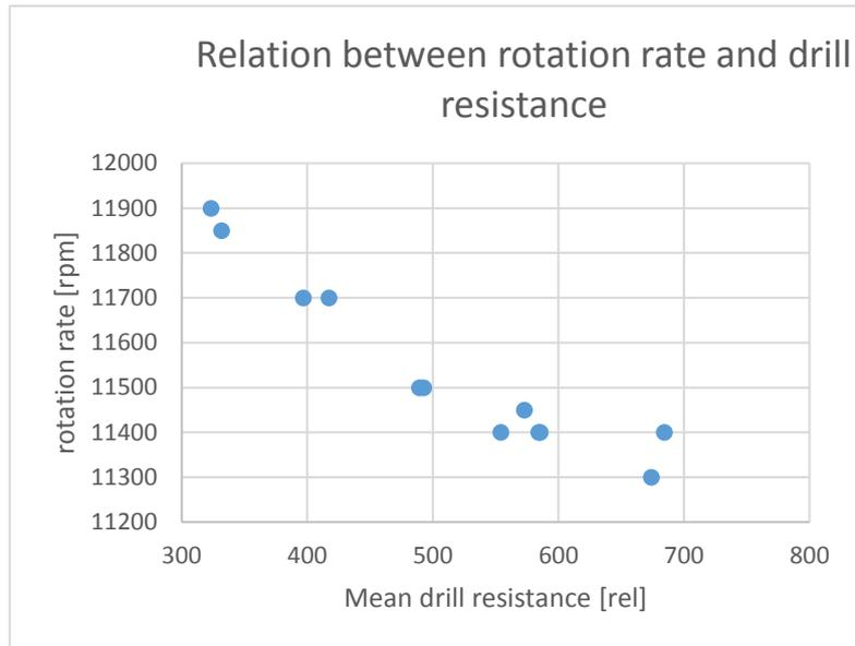
Figure 47 Change of rotation rate with drill resistance; upon drilling sheets of plastic with different densities.
