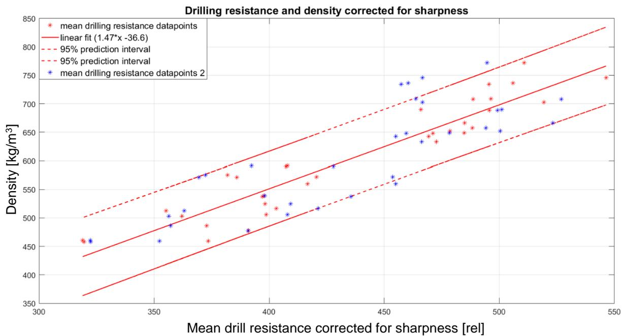
Figure 52 Verification of the regression and prediction interval, data 1 and 2 are the same samples, but drilled with a different drill bit sharpness.
