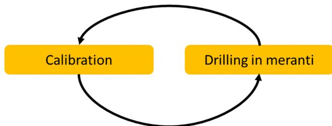
Figure 44 Procedure to test the influence of dulling on the drill resistance.
