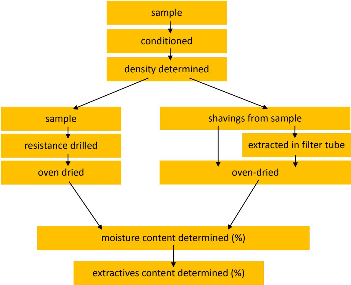
Figure 36 Flowchart of the approach to determine the influence of extractives on the drill resistance
