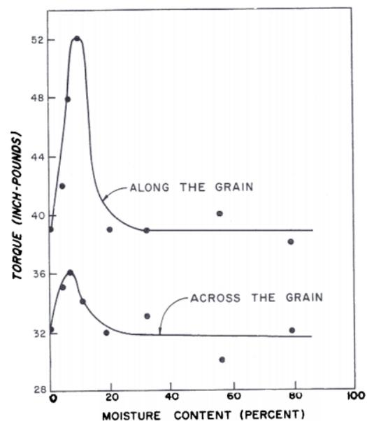
Figure 31 Influence of moisture content on torque upon drilling (McMillin & Woodson, 1972). Along the grain is parallel to the grain whereas perpendicular to the grain is the same as across the grain.
