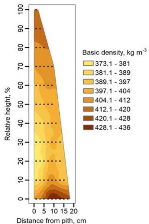
Figure 1 Density variation in a tree trunk (Liepiņš, 2017), note: the pith on the left is the centre of the tree trunk
