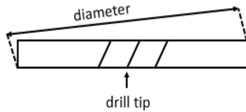
Figure 43 Definition of the drill bit diameter.
