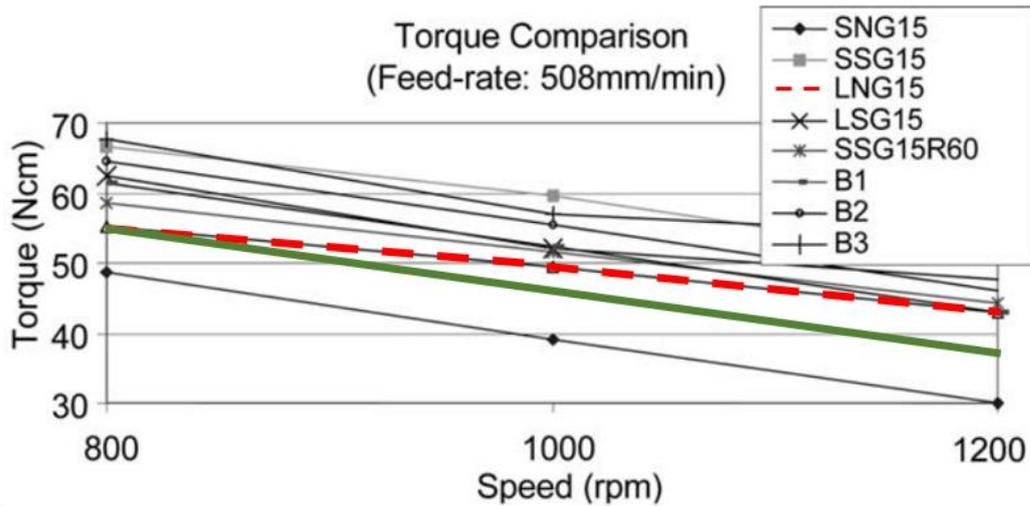
Figure 29 Torque versus rotation rate for a Feed-rate of 508mm/min extended with line of constant specific cutting work (green) adapted from (Zhao & Ehmann, 2002).
