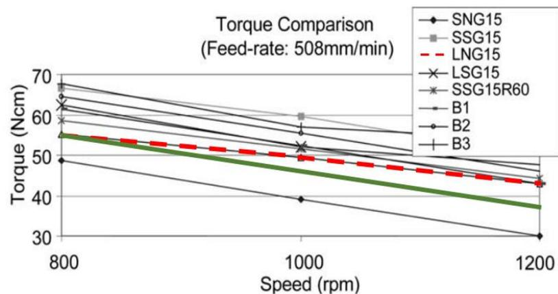
Figure 62 Torque versus speed (green: constant specific cutting work line, red: measurement) adapted from Zhao and Ehmann (2002)
