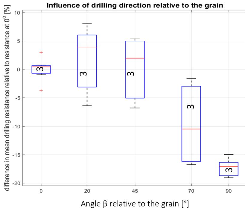
Figure 60 Two conditioned pieces of meranti drilled multiple times at different angles ( $\beta$ ) relative to the grain direction. The numbers indicate the number of measurements in a box.
