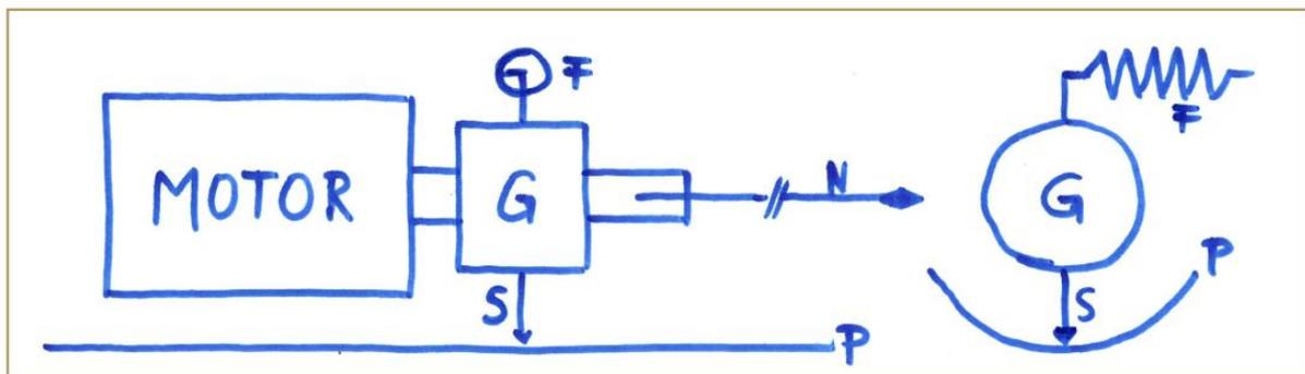
Figure 20 "Sketch of an early resistance drill from 1984: a scratch pin (S) was fixed at a spring (F) loaded gear box (G) between motor and needle (N), creating a 1:1-scaled resistance profile on a wax-paper strip (P)" (Rinn F. , 2012).
