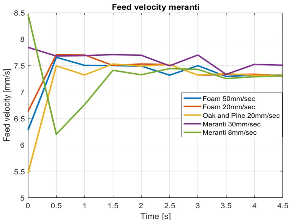
Figure 48 Feed velocity upon drilling different materials. In the legend the feed speed as set on the machine is shown, however this does not influence the actual feed speed as is clearly visible in the graph.
