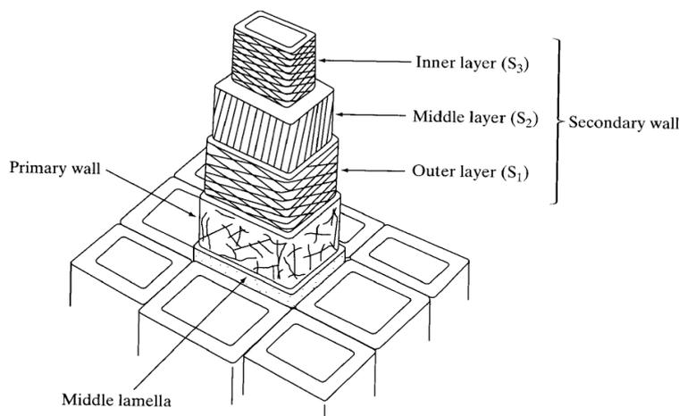
Figure 4 Cell wall schematically (Desch & Dinwoodie, 1996).
