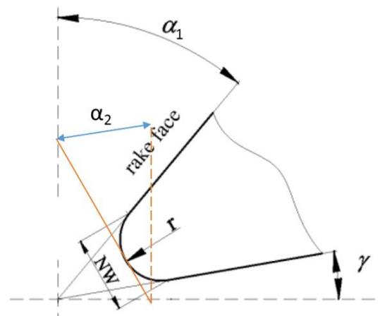
Figure 61 Drill parameters, Clearance angle  $\gamma$ , rake angle  $\alpha_1$ , effective rake angle for a thin chip  $\alpha_2$  and nose width NW adapted from (Cristóvão, 2013)
