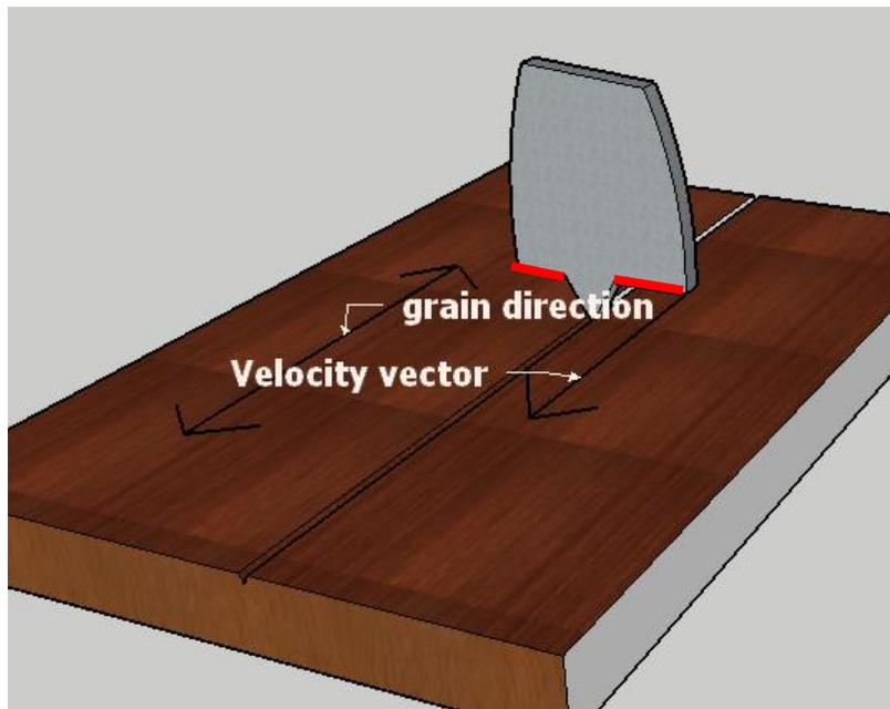
Figure 17 Illustration of the drill bit, indicating the main cutting edge (red), the grain direction and the velocity vector. The velocity vector is drawn at the outer edge; therefore only the tangential velocity is considered, the feed velocity (pointing into the material) is small compared to the tangential velocity and ignored here.
