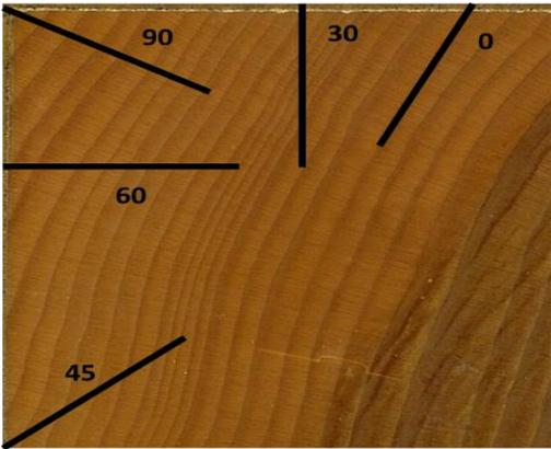
Figure 39 (Transverse plane) drilling direction relative to tangential direction, angles  $\theta$  represent the angle relative to the tangential direction (tangential direction means parallel with the growth rings).
