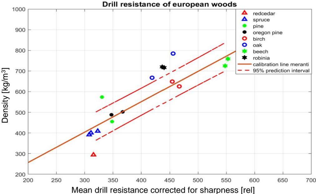
Figure 54 Drill resistance of conditioned European woods plotted with the calibration line and prediction interval of meranti. Each mark in the graph represents one sample, and is the mean drill resistance of multiple (usual three) drillings in that sample.
