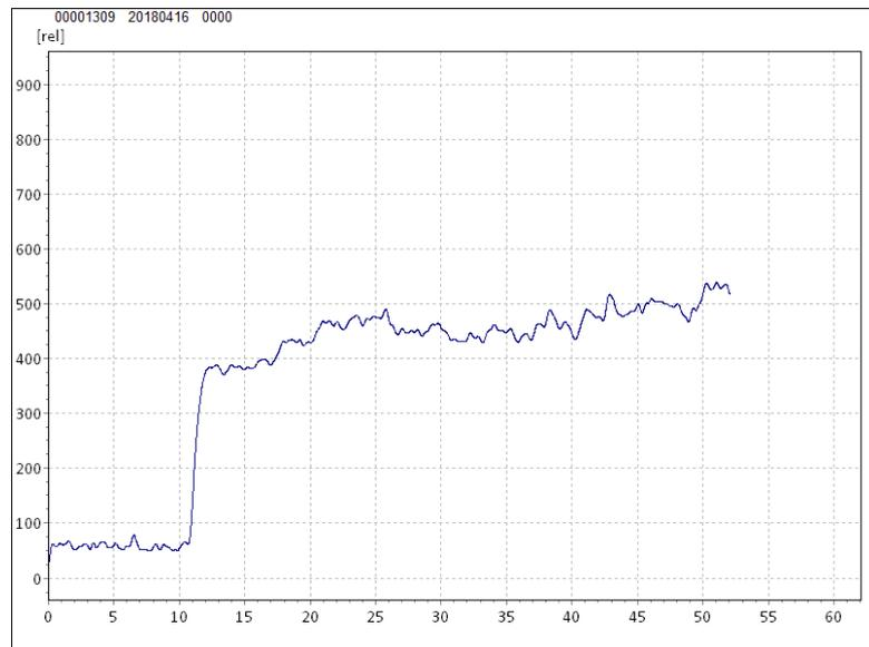
Figure 34 Typical Resistograph resistance profile with depth at the x-axis and drill resistance, measured relative to the idle speed on the y-axis.
