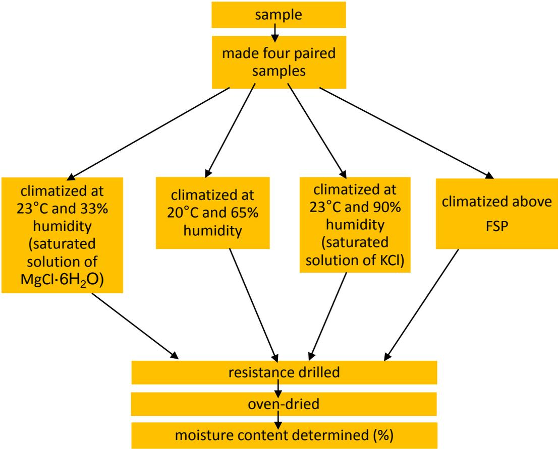
Figure 37 Flowsheet showing the approach used for the determination of the influence of moisture content on the drill resistance.
