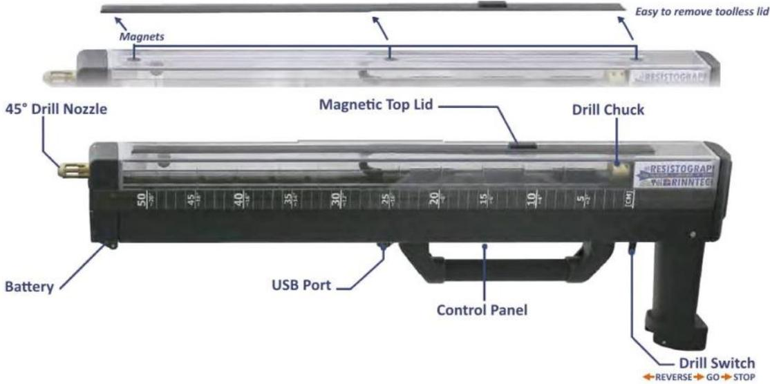
Figure 33 Figure showing all the different components of the Resistograph drill (Rinntech, 2014).
