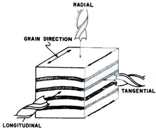
Figure 32 definition of radial, tangential and longitudinal drill direction according to Woodson and McMillin (1972)
