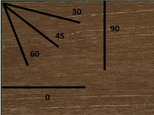
Figure 40 (Radial or tangential plane) drilling direction relative to the grain shown are the angles  $\beta$  where  $0^\circ$  is parallel to the grain and  $90^\circ$  perpendicular to the grain.
