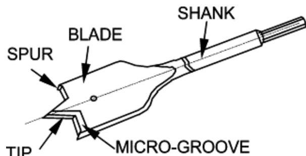
Figure 24 The spade drill bit (Zhao & Ehmann, 2002).
