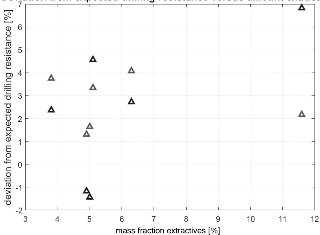
Figure 55 Influence of mass fraction extractives (% of dry mass) on drill resistance for meranti each datapoint is the mean drill resistance of one drilling in a sample.
