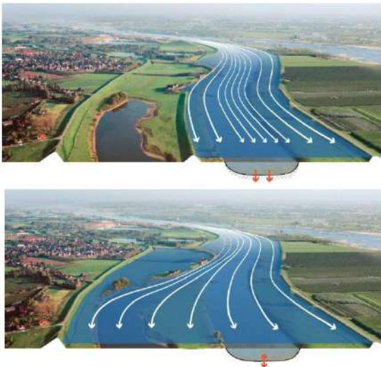
Figure 1. Principle of the multi-channel concept. By widening the wetted perimeter, the energy is better divided through summer and winter bed.
