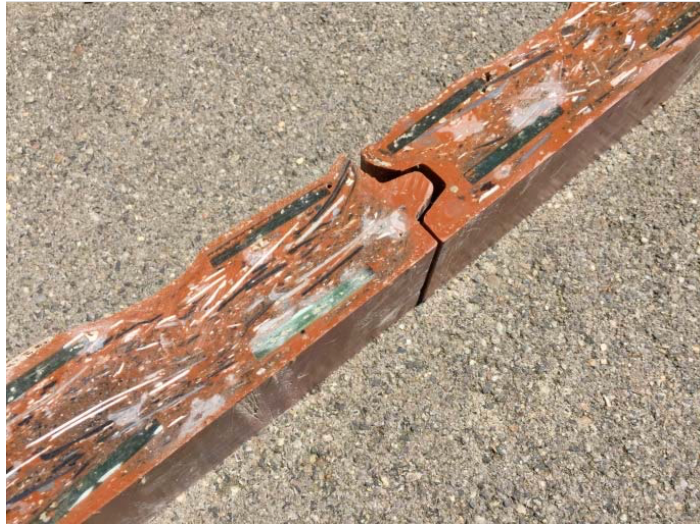
Figure 8-3: Section of the sheet piling walls with fragments and flakes of EoL composites as reinforcement, produced by Windesheim (Ten Busschen, 2018).
