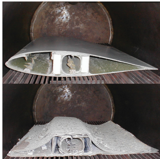
Figure 9-3: a) The before and b) after look of a part of a WTB treated in a pyrolysis reactor (picture courtesy of ReFiber; Larsen, 2009).
