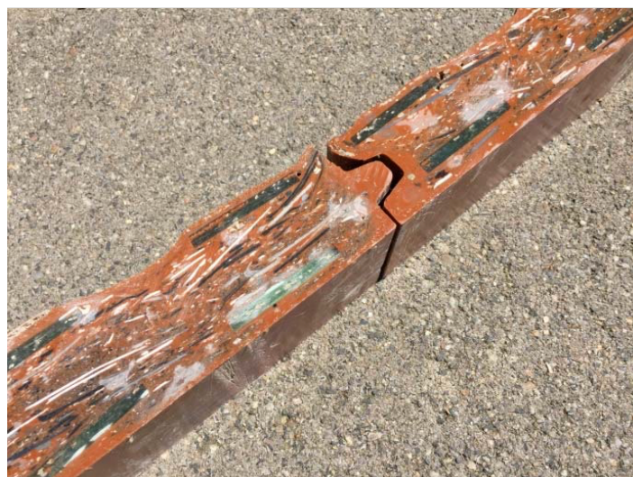
Figure F-2: Section of the sheet piling walls with fragments and flakes of EoL composites as reinforcement, produced by Windesheim (Ten Busschen, 2018).
