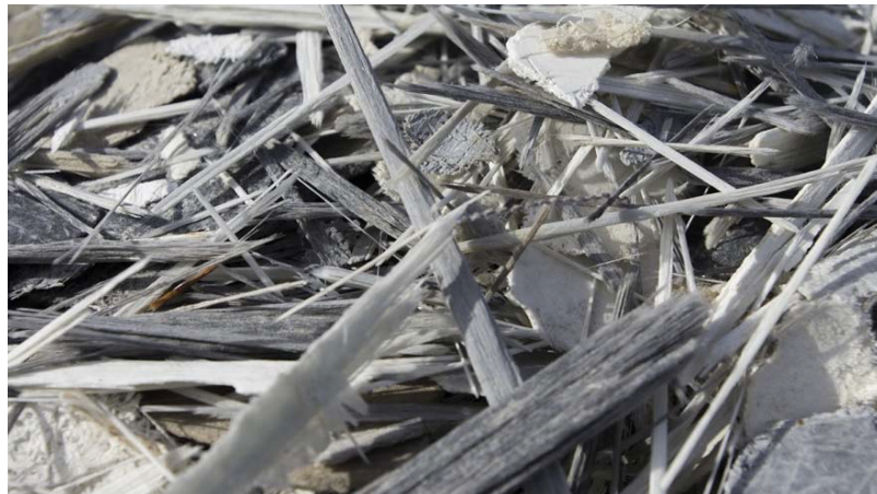
Figure F-1: Strips and flakes of EoL composite material from WTB and boat hulls used as reinforcement in new composite material (Ten Busschen, 2018).
