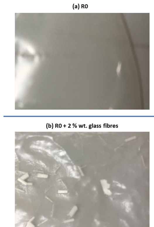
Figure 93: 0% ceramic filler loading sample without (a) and with (b) glass fibres
