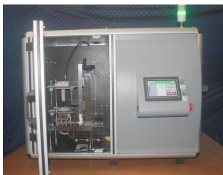
Figure 42: Corona poling unit
