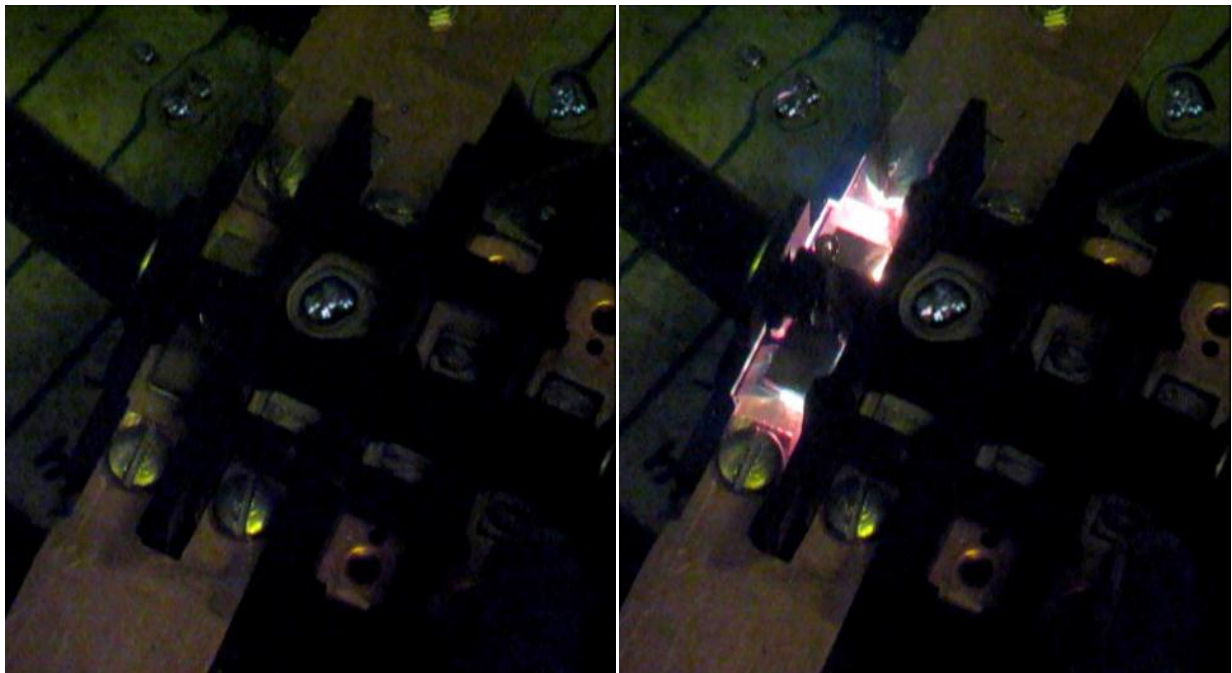
Figure 3.9 : Arc as seen in the laboratory setup for arcing.
