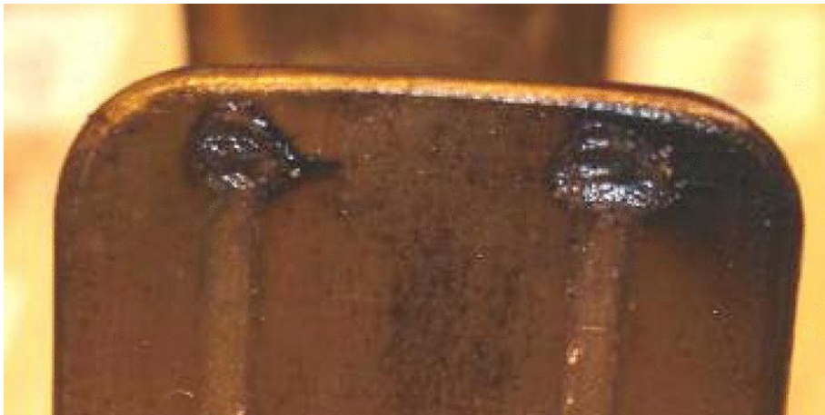
Figure 2.10: Showing the damage to the coarse selector contacts due to the long term degradation effects [19].
