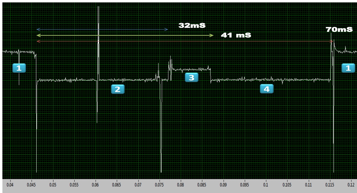
Figure 4.7 : DRM graph obtained from an actual 3 phase, motor and spring actuated tap changer.
