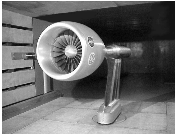
Figure 3.4: NASA's Glenn UHBPR engine 1:5 scale model, from [40].
