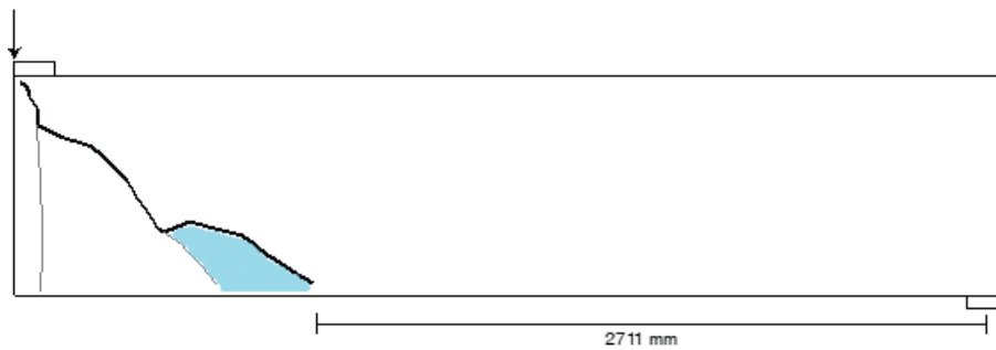
Fig. 5.4.1 Critical crack for H352
