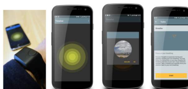
Figure 2.5 From top left to right: (a) Sensor wristband with TimeOut in the background; (b) main screen showing continuous visualization of EDA; (c) prompt for intervention; (d) one of five tasks in the behavioral intervention protocol (Flobak et al, 2018).
