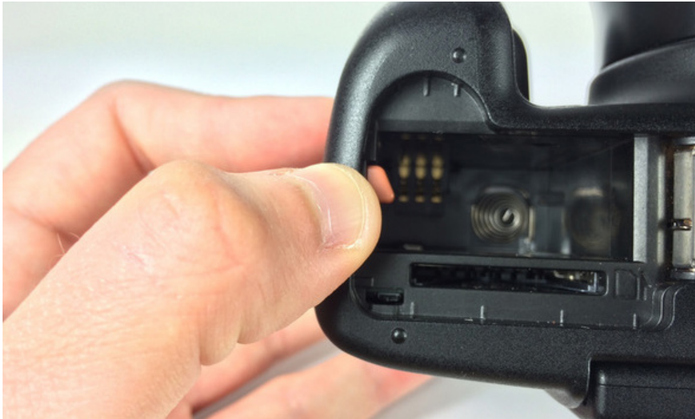
Figure 28.7: A photo of the battery engage and release in a Canon camera. The brown latch keeps the battery in place. When rotated, the battery is sprung up by the spring at the bottom of the camera. Making it easy for the user to change batteries (Rund, 2015).
