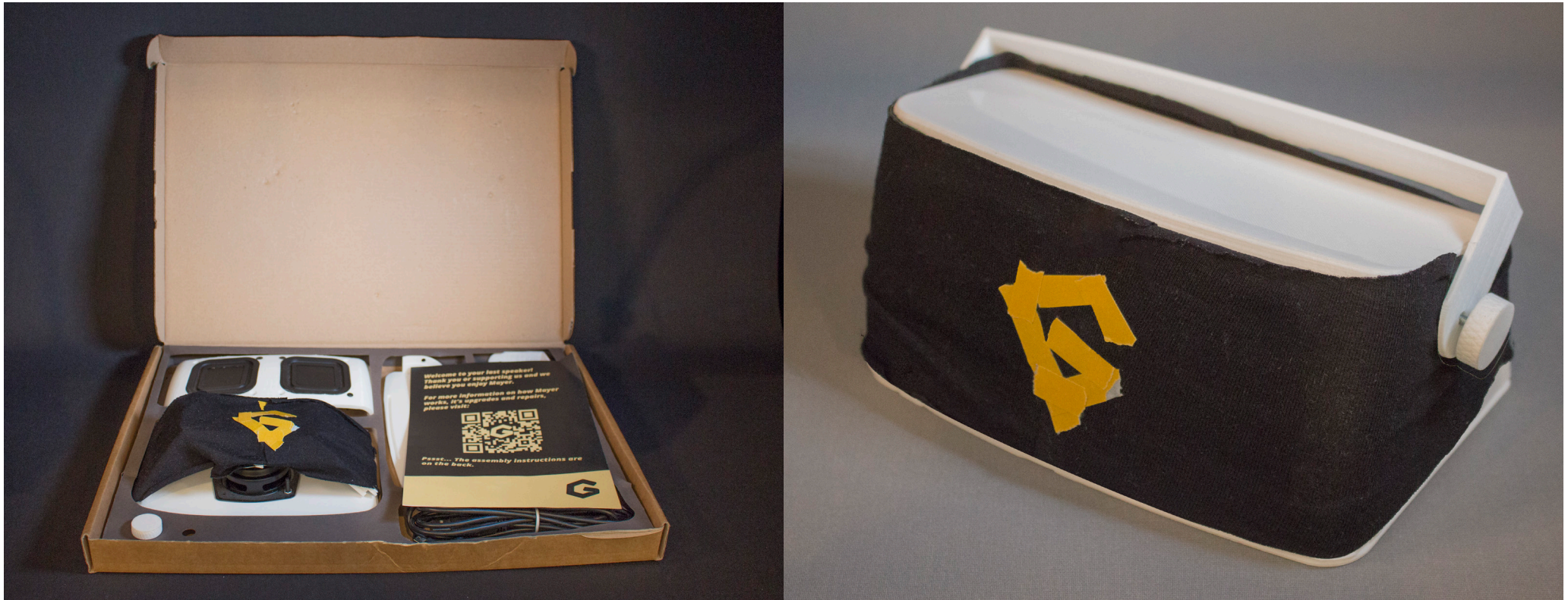
Figure 30.2: The left photo is of the postal box containing the prototype for the assembly test. The box contains the bottom with the sides, the top, the front and the back of the speaker, together with a mini-USB cable and a manual. The photo on the right is the prototype assembled.
