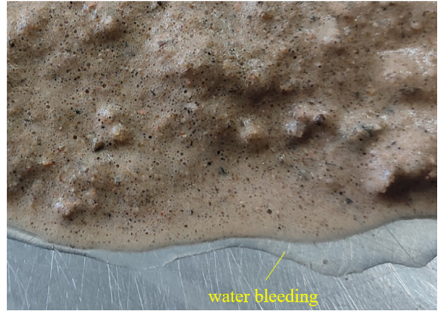
Fig. 17. Periphery of the sand specimen with w = 15\% and FIR = 50\% .
