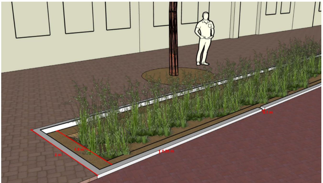
Figure 46: Example of the dimensions of a Bioswale implemented in the Tweede Atjehstraat
